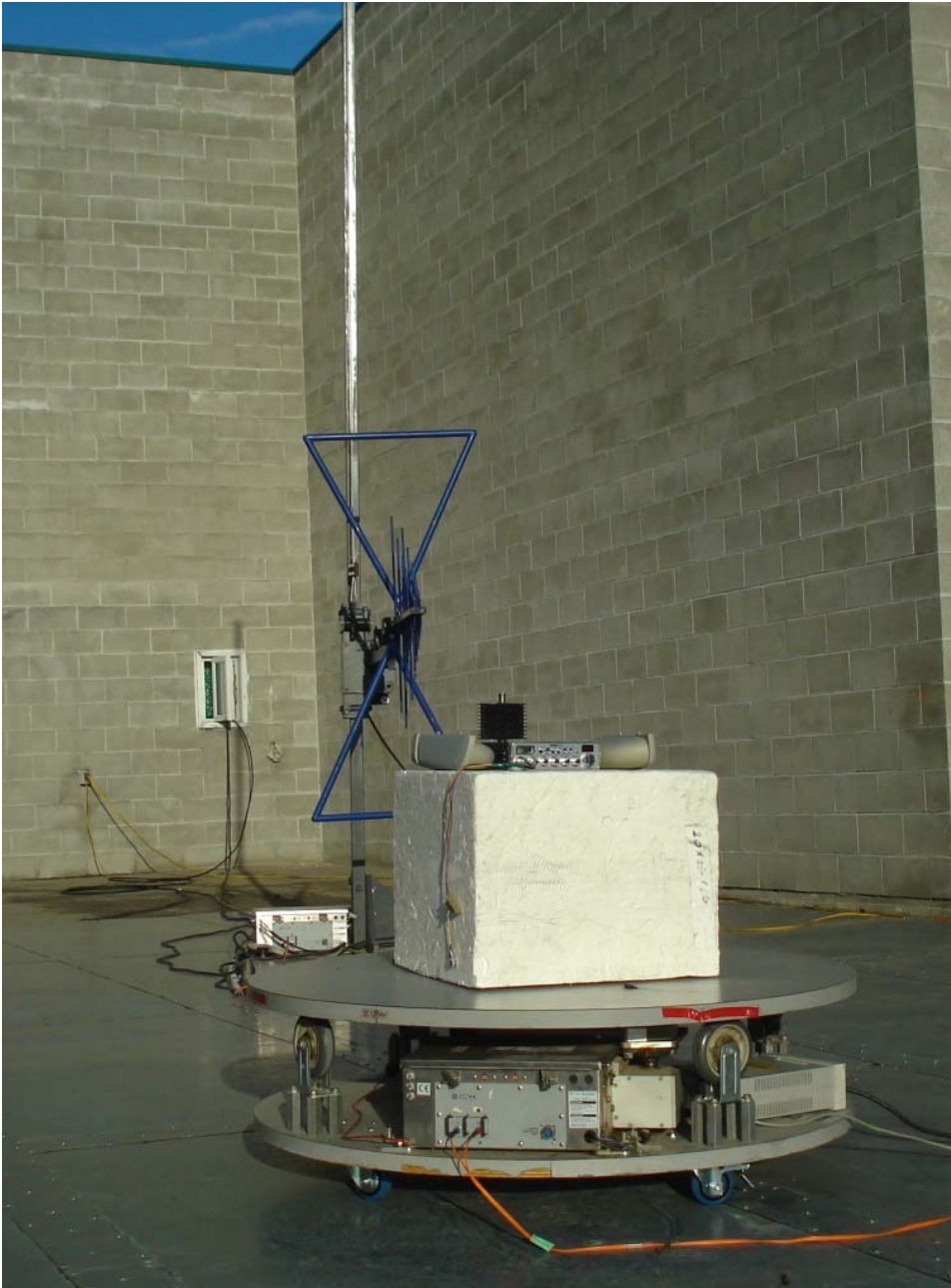
P1 – Radiated Emission on OATS
