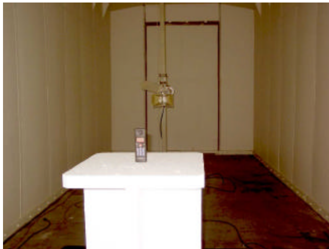
Uniden - Handset Testing Peak Power Spectral Density - Radiated
