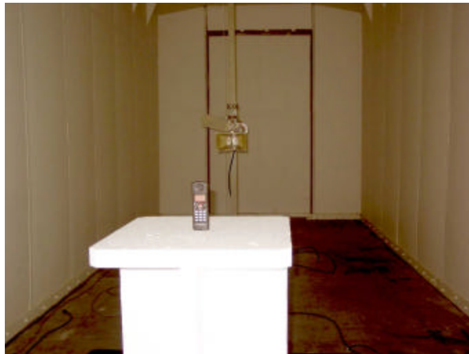
Uniden – Handset EIRP Measurement at OATS
