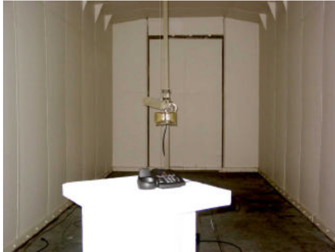
Uniden - Base unit Testing Peak Power Spectral Density - Radiated
