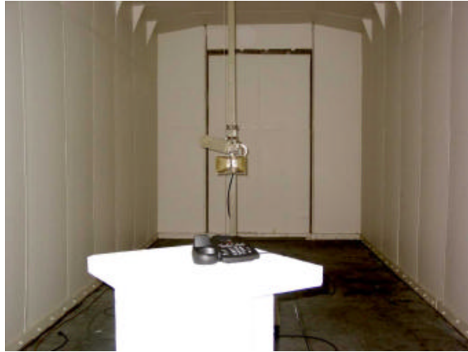
Uniden – Base Unit EIRP Measurement at OATS
