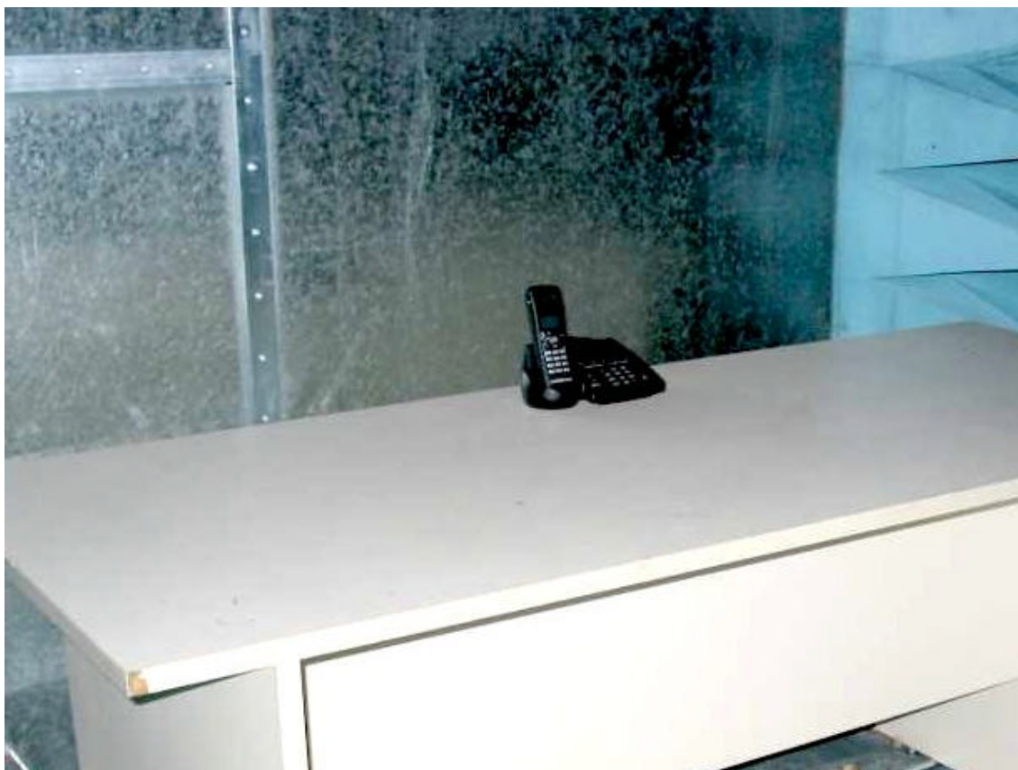
Testing Conducted Emissions on Power Lines Handset and Base unit connected to LISN Frequency range: 450 kHz – 30 MHz
