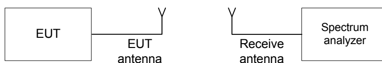
Figure 7.2.1 Occupied bandwidth test setup
