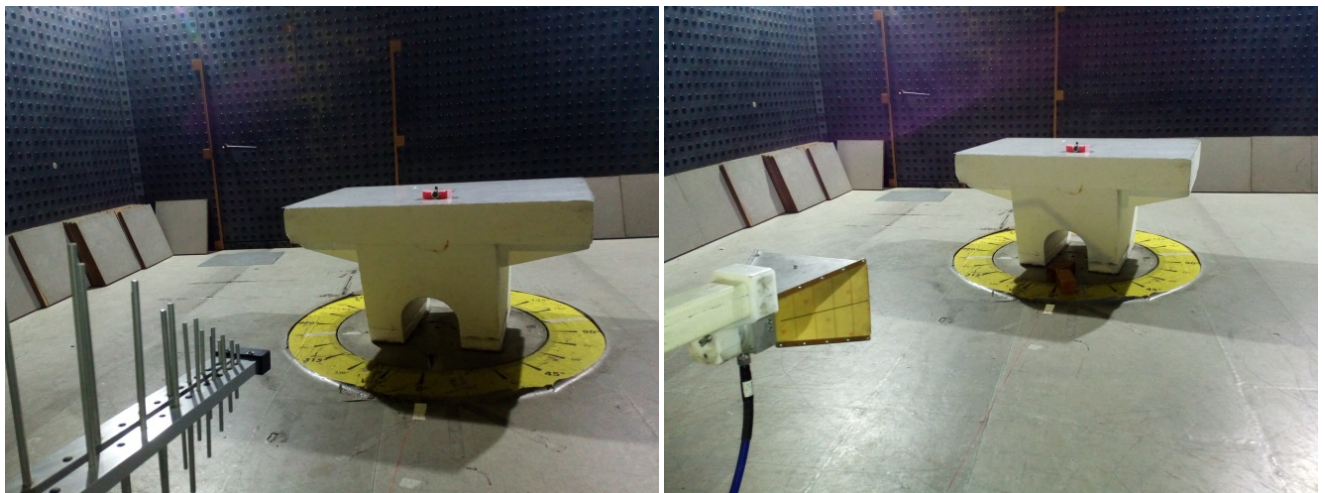
Photograph 8.1.1 Setup for radiated emission measurements
