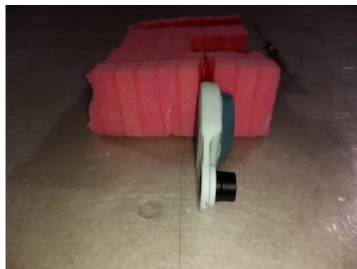
Photograph 6.4.3 EUT in Z-axis orthogonal position
