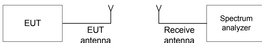
Figure 7.4.1 Occupied bandwidth test setup
