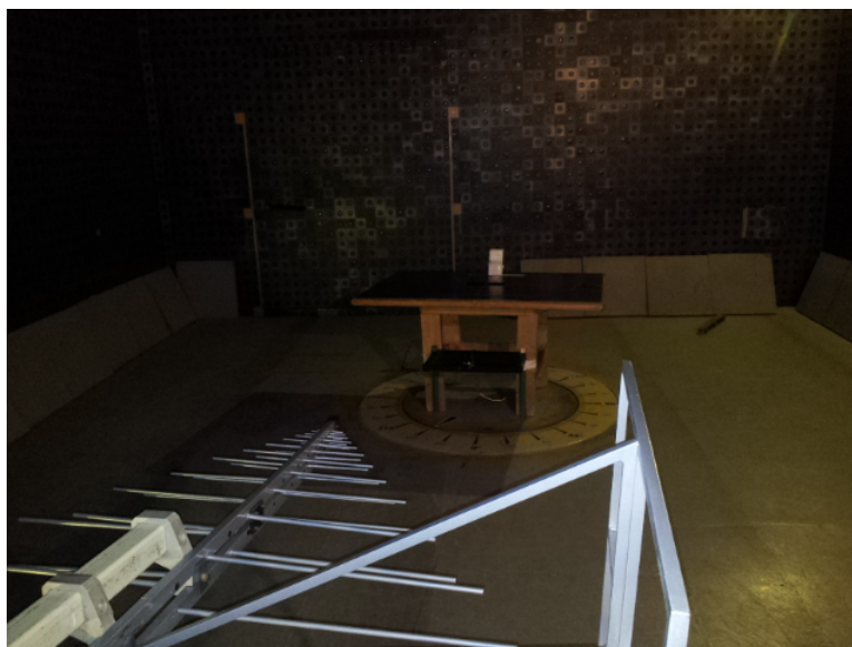
Photograph 8.1.1 Setup for radiated emission measurements
