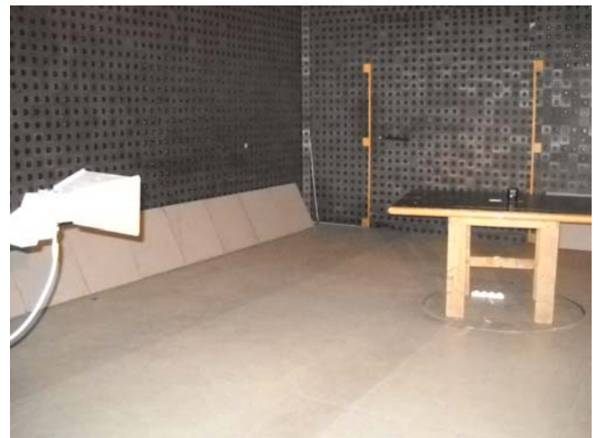
Photograph 8.1.1 Setup for radiated emission measurements
