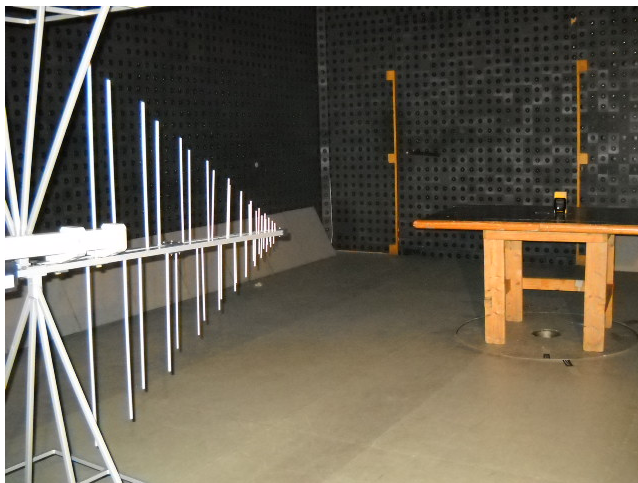
Photograph 8.1.1 Setup for radiated emission measurements
