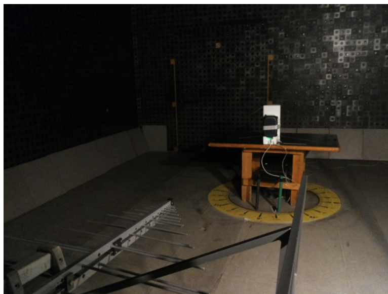
Photograph 8.1.1 Setup for radiated emission measurements
