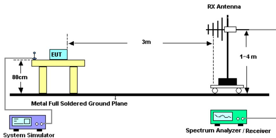
For radiated test above 1GHz
