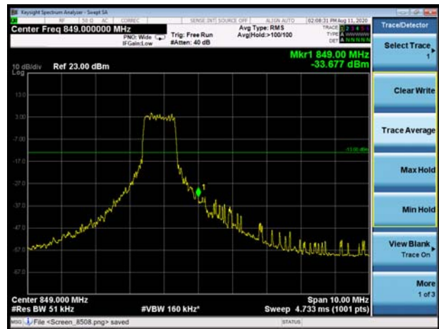
LTE Band 26 QPSK 1.4MHz CH-High 1RB
