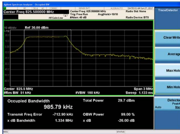
LTE Band 26 16QAM 3MHz CH-Middle
