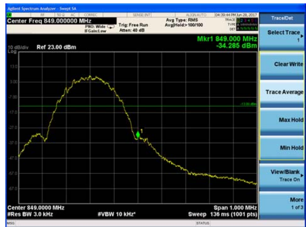
LTE Band 5 QPSK 1.4MHz CH-High 1RB
