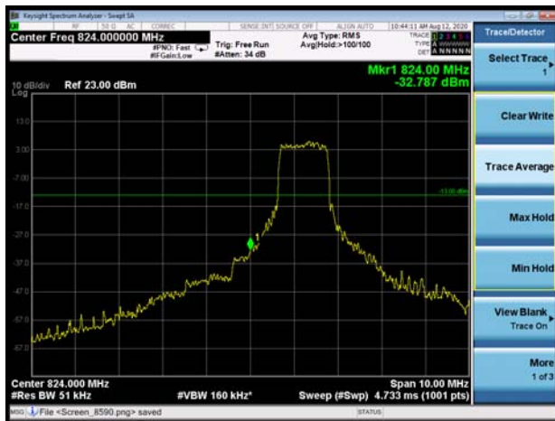
LTE Band 26 QPSK 10MHz CH-Low 100%RB
