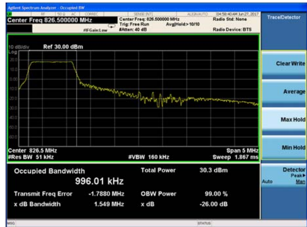
LTE Band 26 16QAM 5MHz CH-Middle
