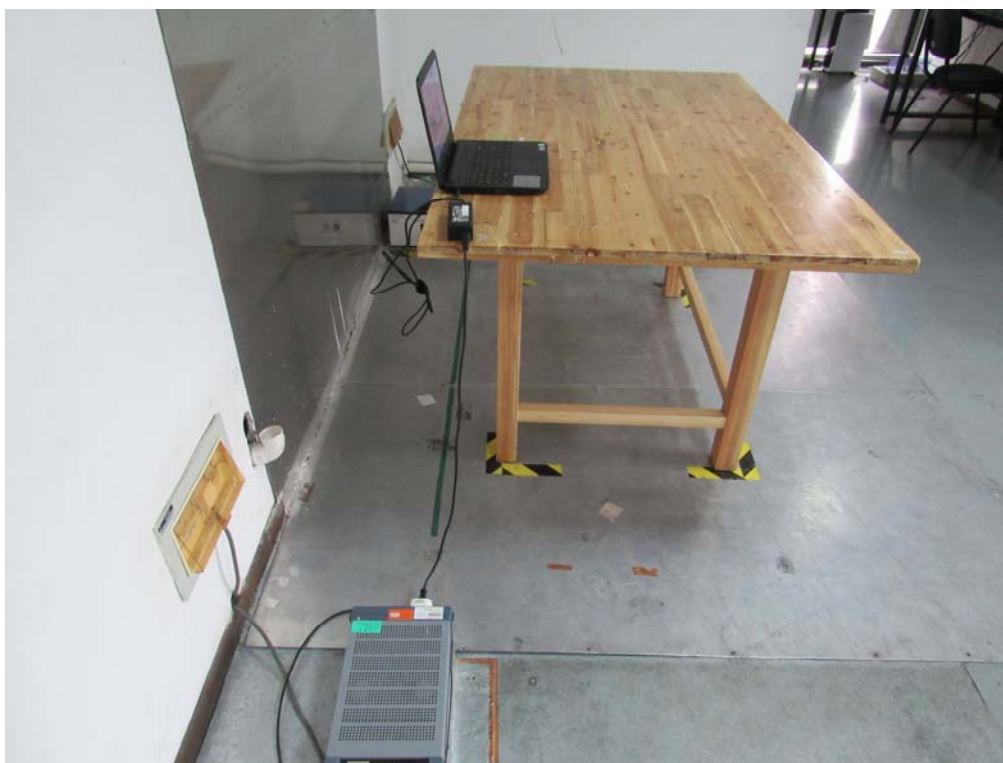
Conducted Emissions Setup Side View
