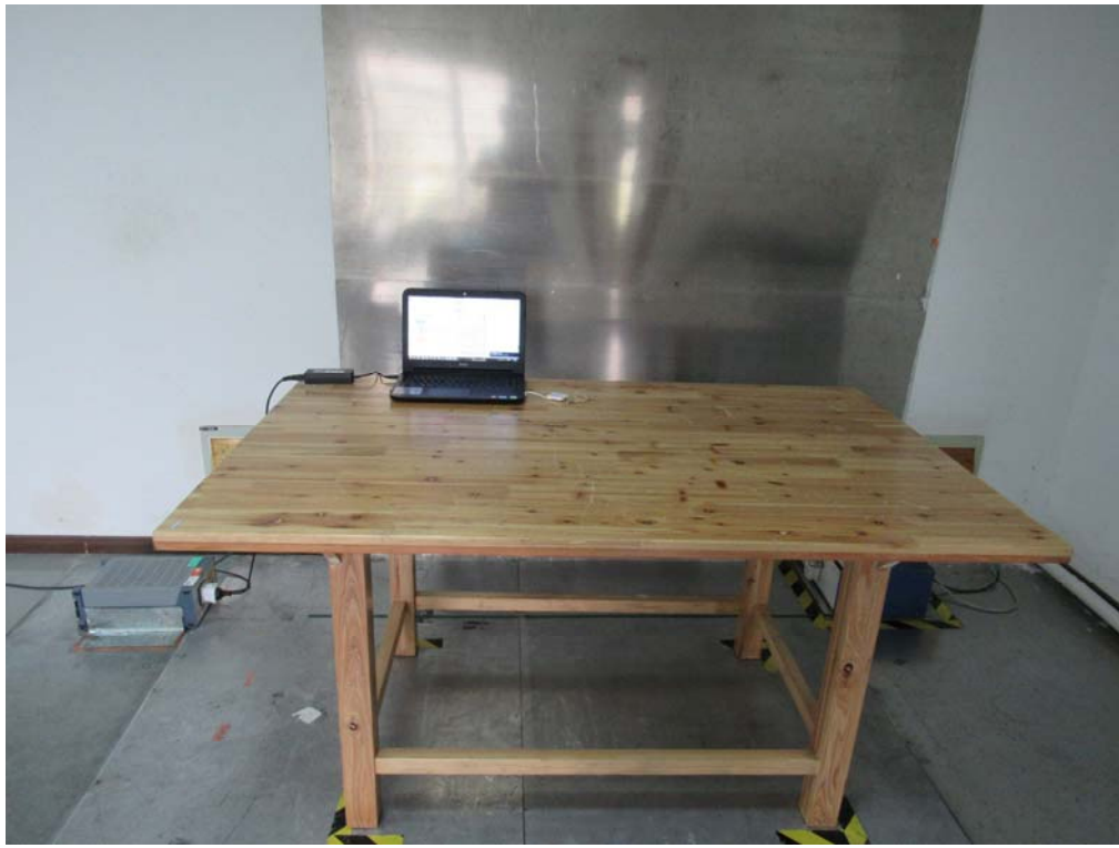
Conducted Emissions Setup Front View
