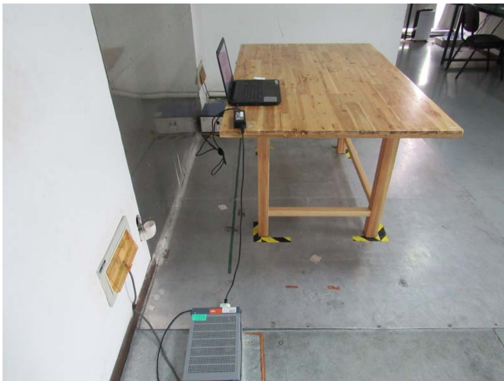
Conducted Emissions Setup Side View
