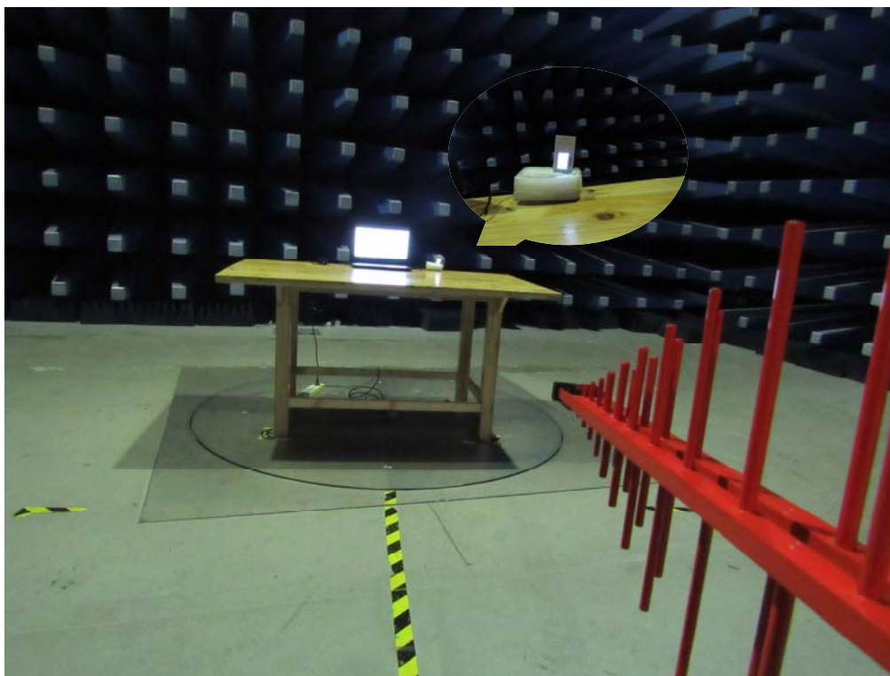
Radiated Emissions Setup Below 1GHz Front View
