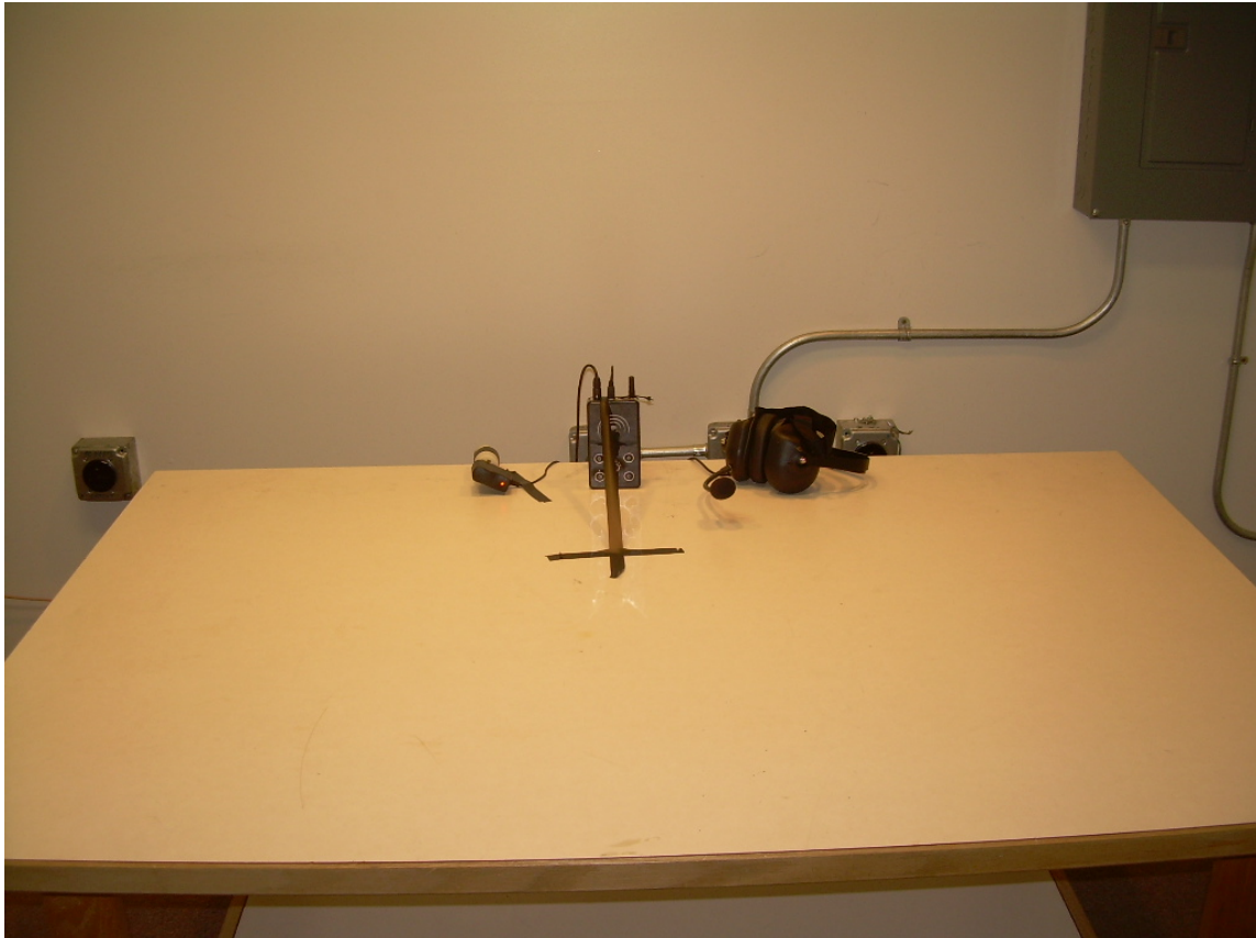
Photograph 3 – Front View Conducted Disturbance Worst Case Configuration
