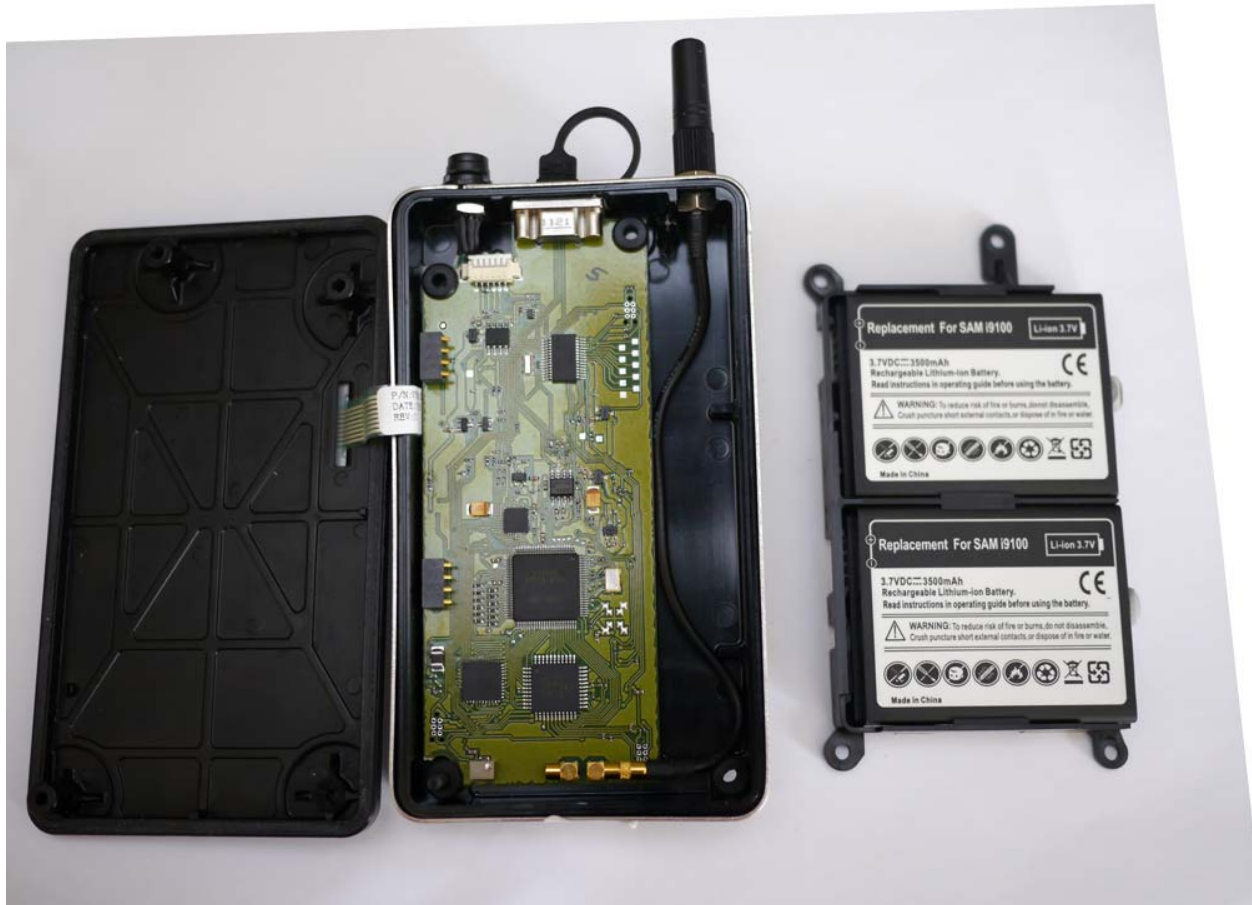
Photograph 10 – View of the EUT Housing Open with Batteries Removed Showing Front Side of the PCB
