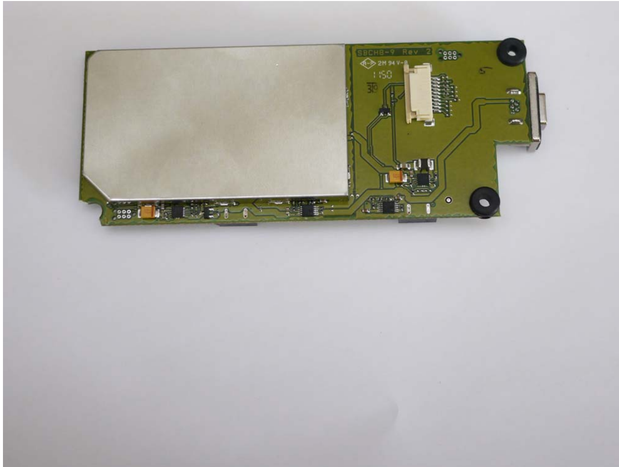
Photograph 12 – View of the Bottom of the PCB with RF Shield in Place
