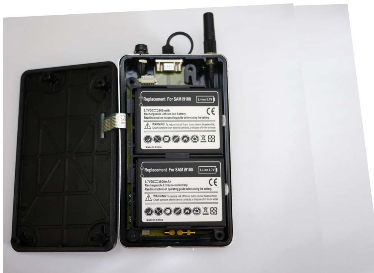
View of the EUT with Housing Opened
