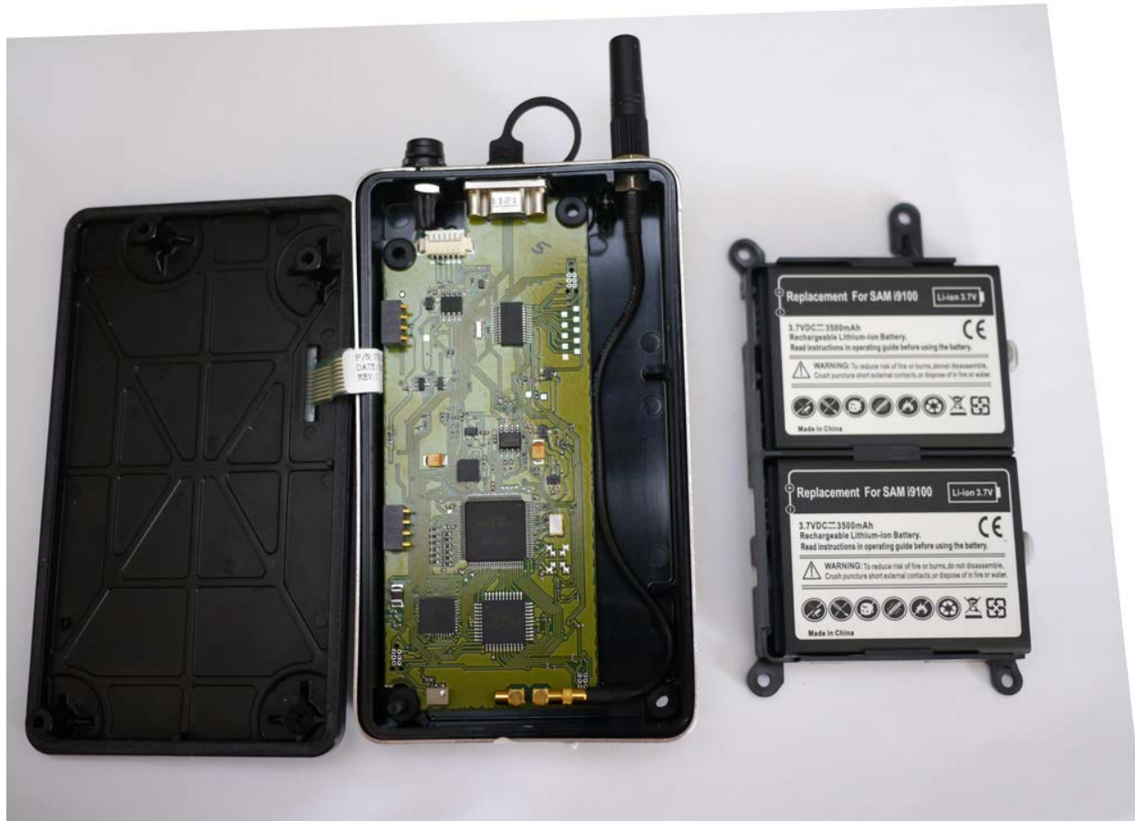
View of the EUT Housing Open with Batteries Removed Showing Front Side of the PCB
