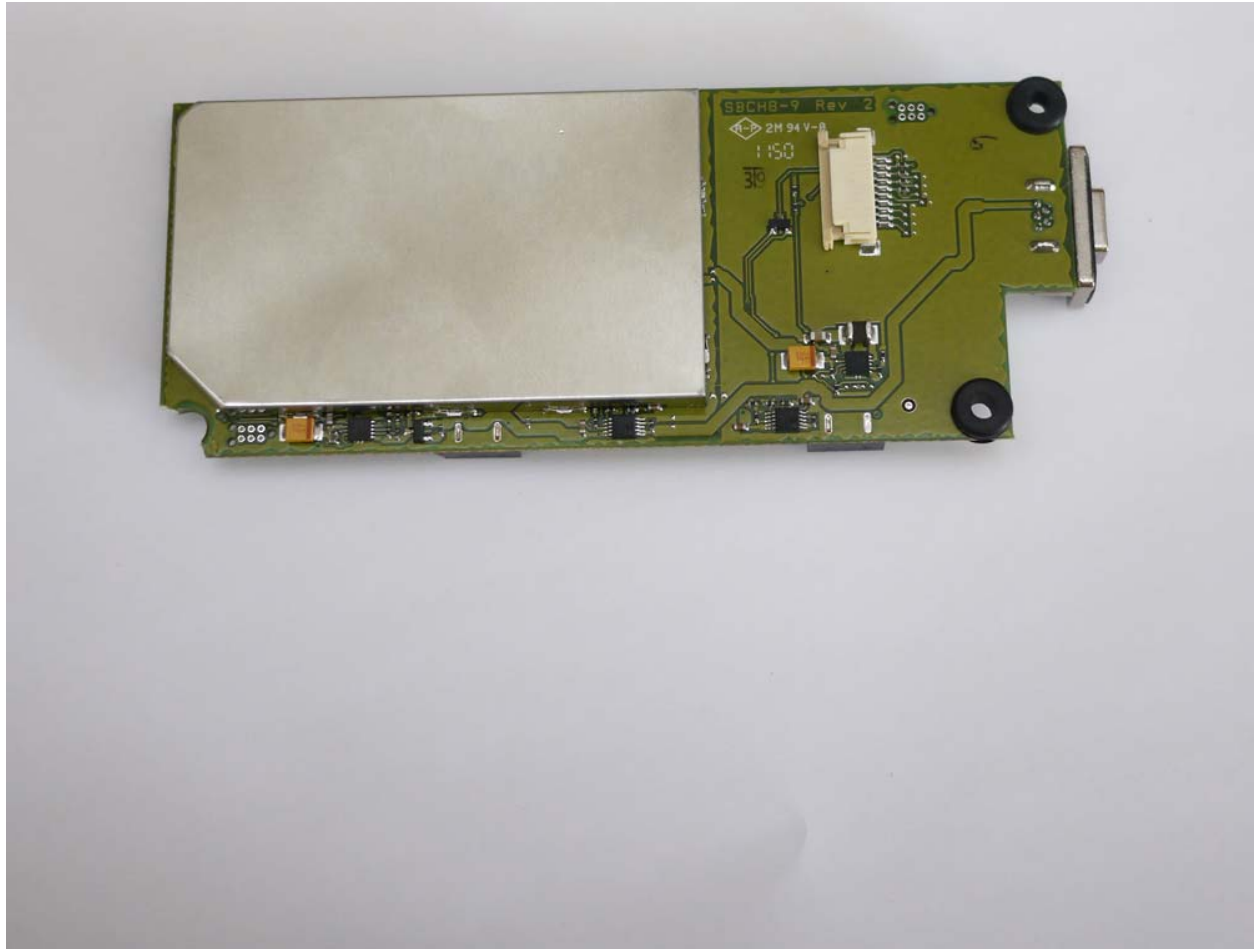
View of the Bottom of the PCB with RF Shield in Place
