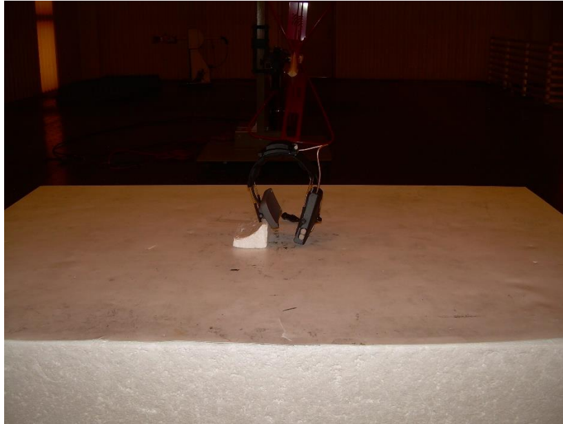
Photograph 1: View Radiated Emissions Worst-Case Configuration – Vertical
