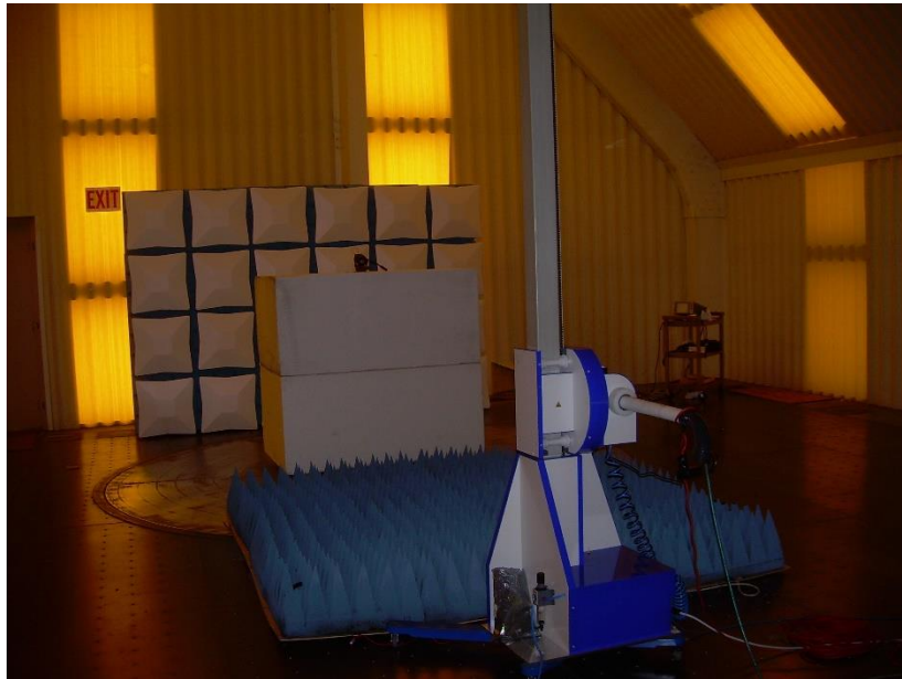
Photograph 4: Front View Radiated Emissions Worst-Case Configuration – Above 1000 MHz
