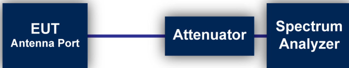
Figure 1: Direct Connection at the Antenna Port Test
