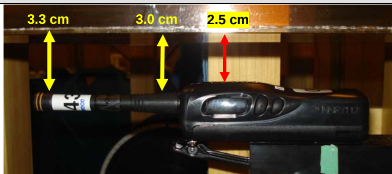
Face-held SAR Configuration - Antenna 3, Battery a
