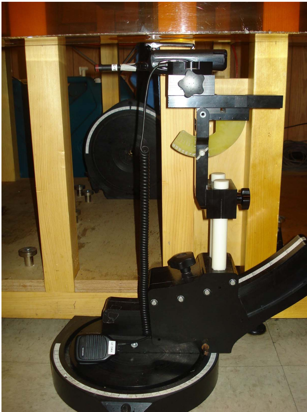
Body-worn SAR Configuration Test Setup
