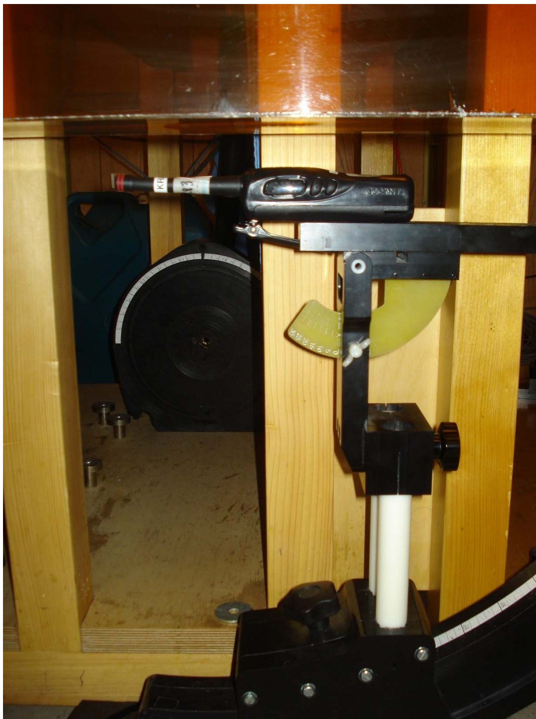
Face-held SAR Configuration Test Setup
