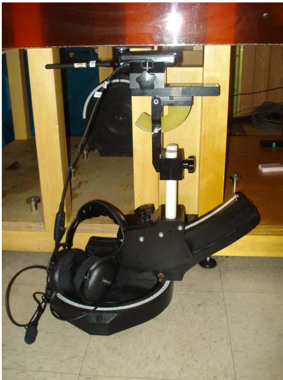
Body-worn SAR Configuration - Antenna 7, Battery a, Audio G3b
