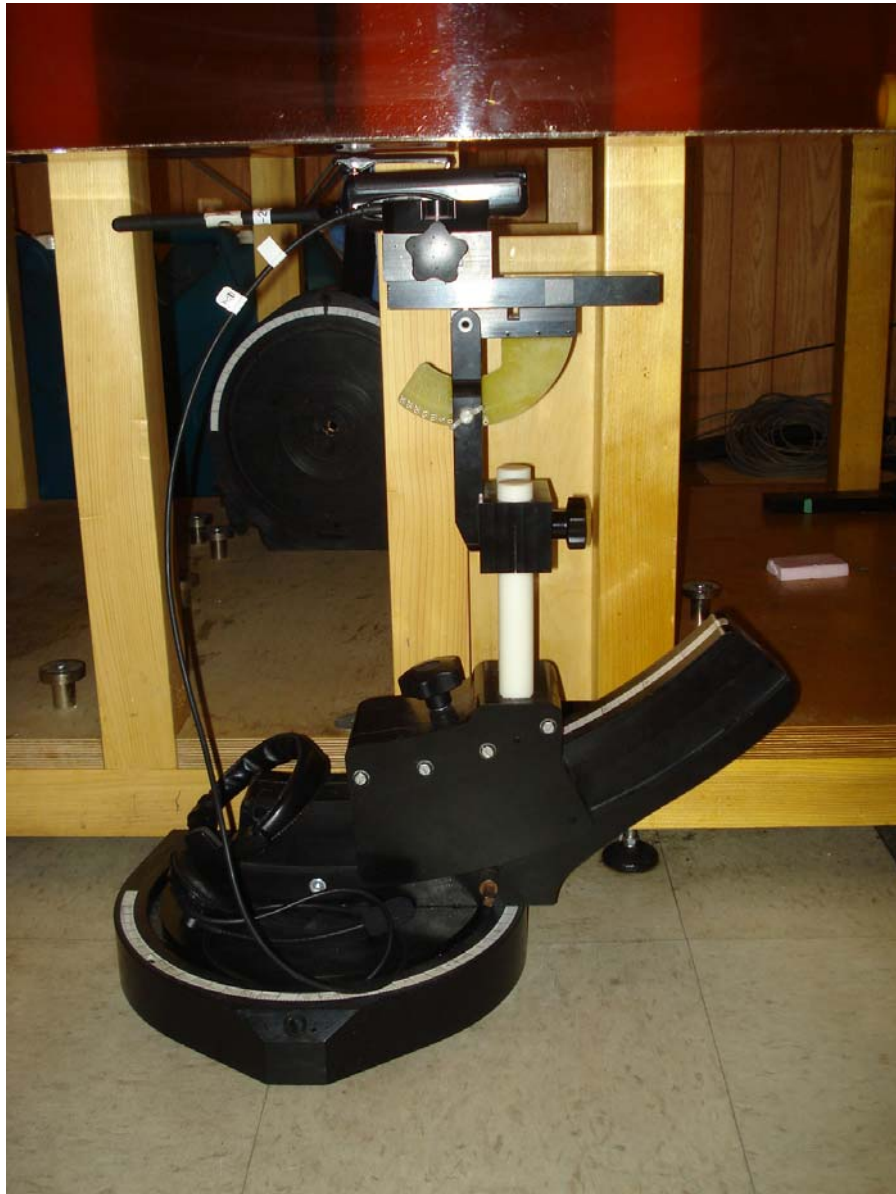
Body-worn SAR Configuration - Antenna 7, Battery a, Audio G2b
