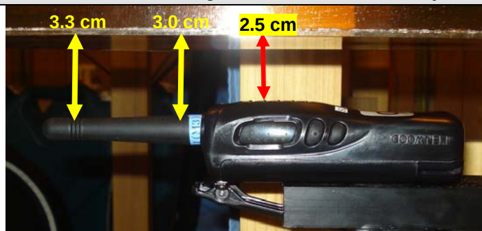
Face-held SAR Configuration - Antenna 12, Battery a
