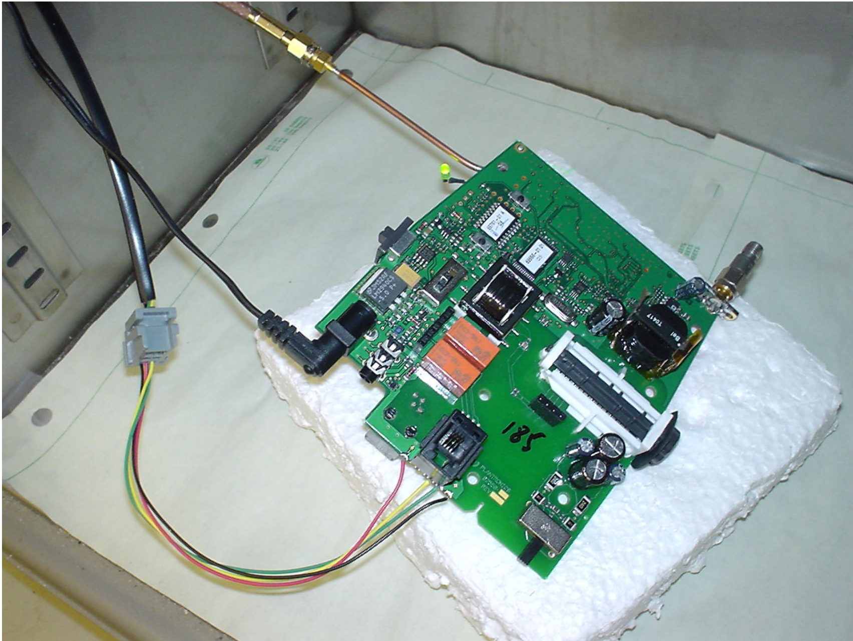
Fig. 43 - Interconnection between the base EUT and the test system; RF conducted connection, DC power supply, and control/communications bus for administrative commands
