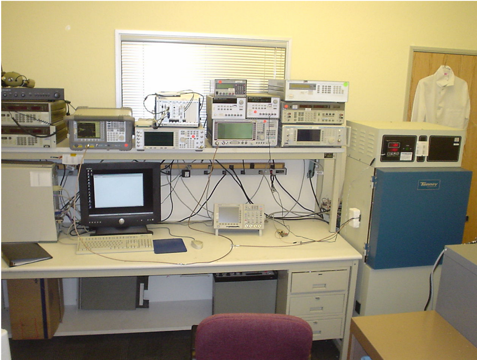
Fig. 41 - View of test system configured for the tests of clause 6.2.1 for the base EUT. EUT is in the temperature chamber at right. EUT power supply is top right-center. EUT RF cabling is connected as described in the text, to the CMD60 analyzer and the E4407B spectrum analyzer. The controller interface circuit (RS232 to CMOS levels) can be seen lower right-center.
