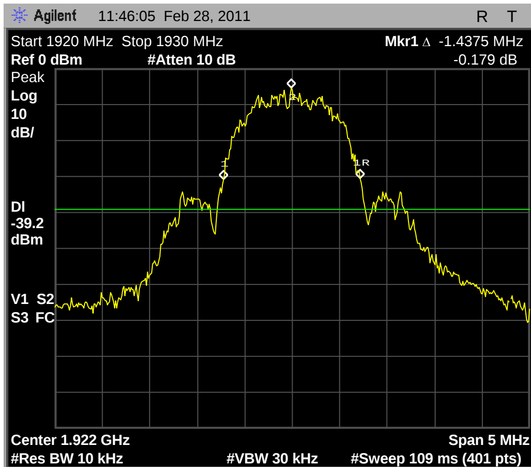
Fig. 67 - Base EUT in low power WBM, 1.4375MHz emissions bandwidth on low carrier; vs. 1.435MHz in max power normal mode.
