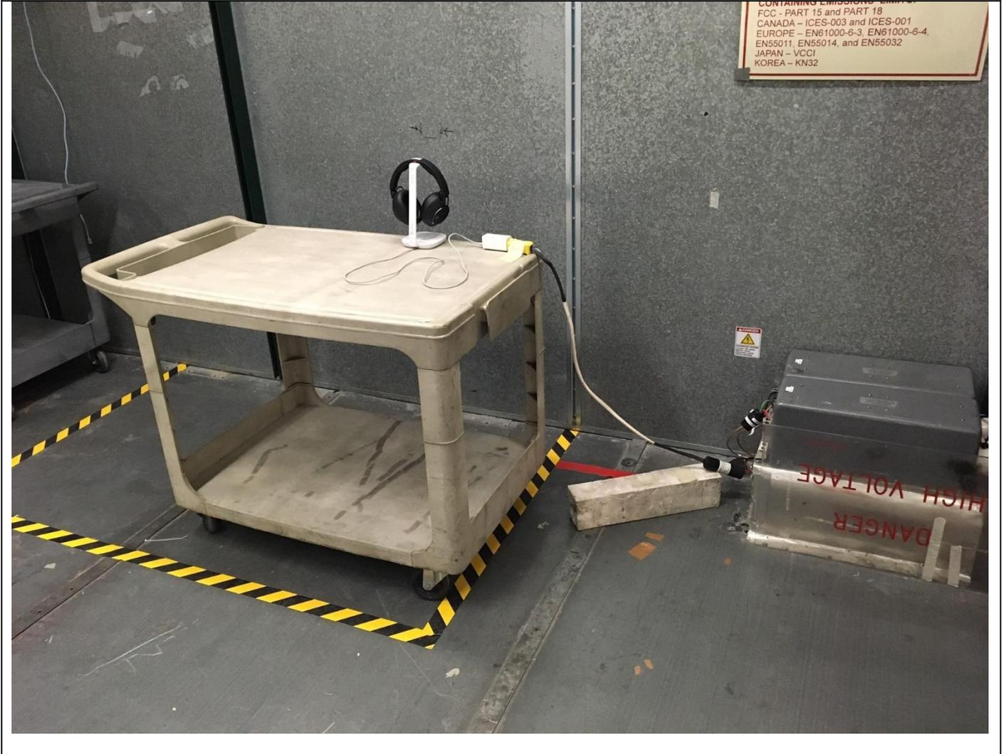
**Photo of test setup for Mains Conducted Emissions Configuration 2, operating mode 2**
