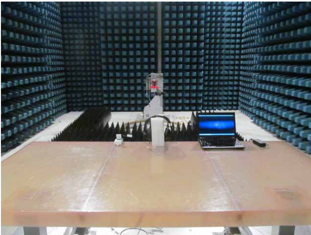
Description: Radiated Emission Test Setup for 1~18GHz
