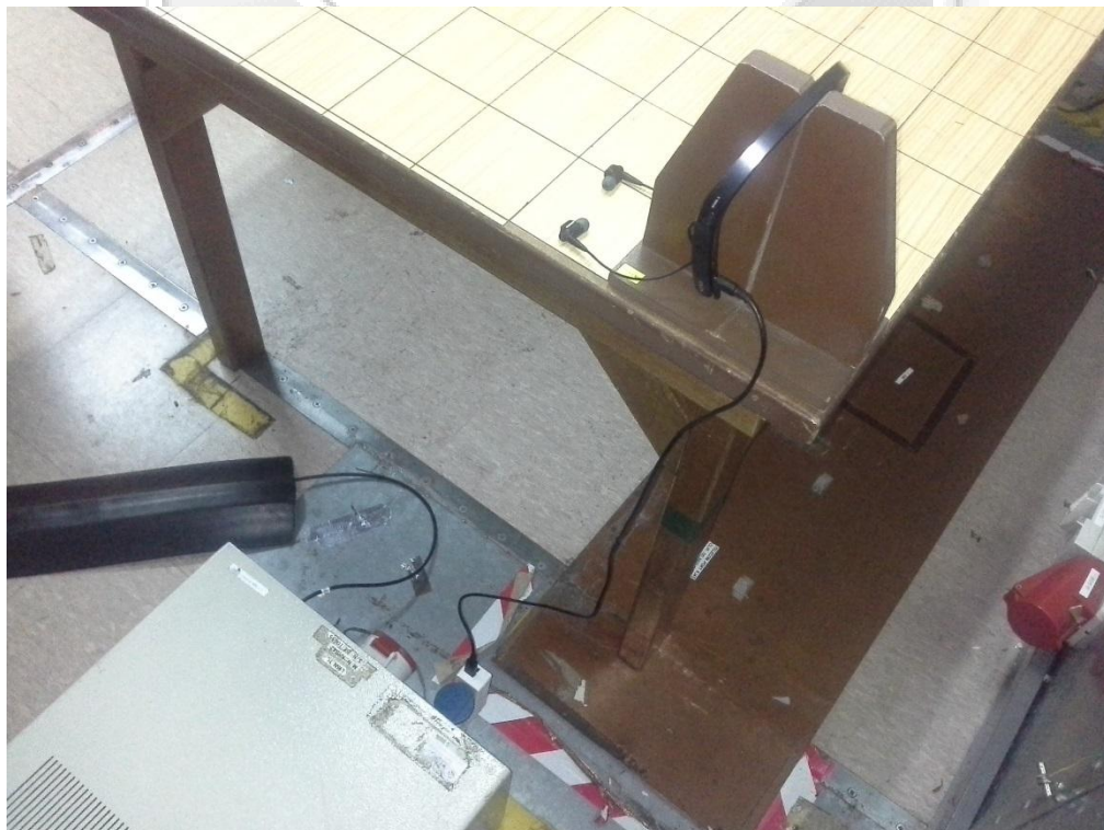
Conducted Emissions Test Setup (Rear View)
