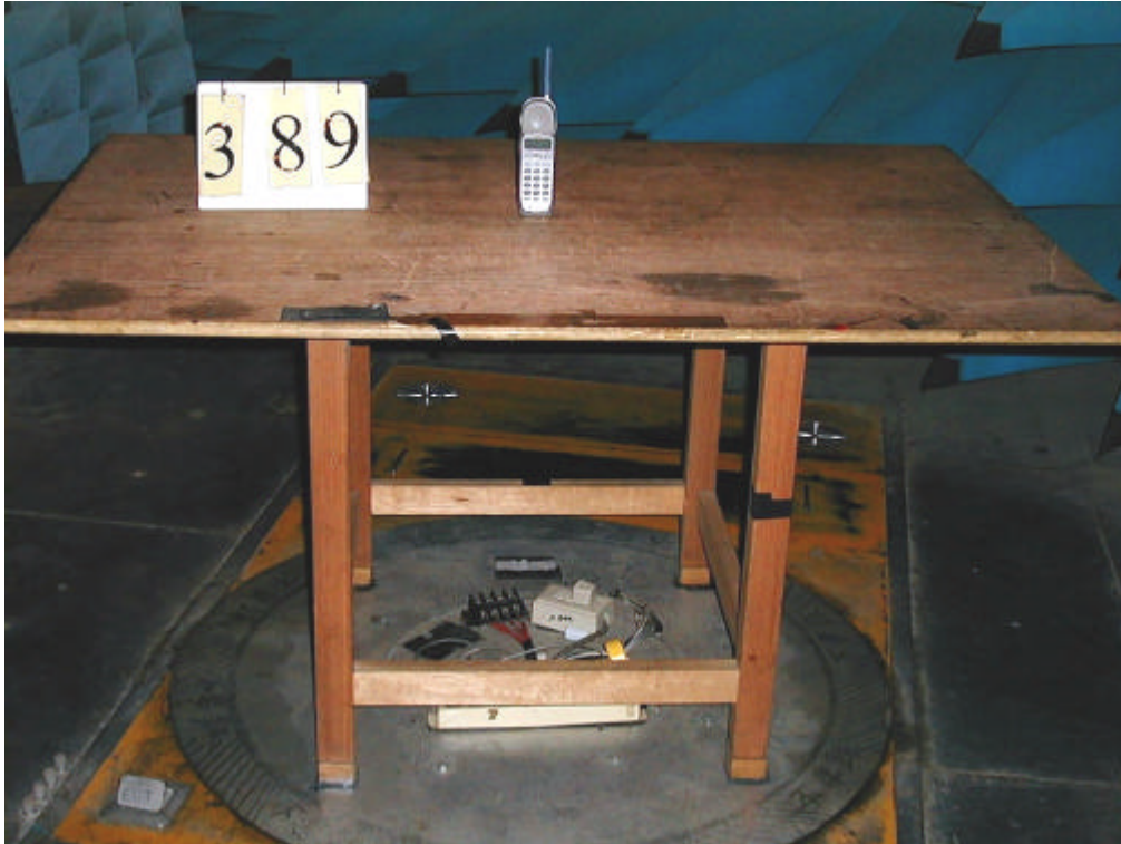
Pig 1 Front View of the Test Configuration (HANDSET)
