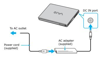
2 Plug the power cord into the AC adapter and an AC outlet.
