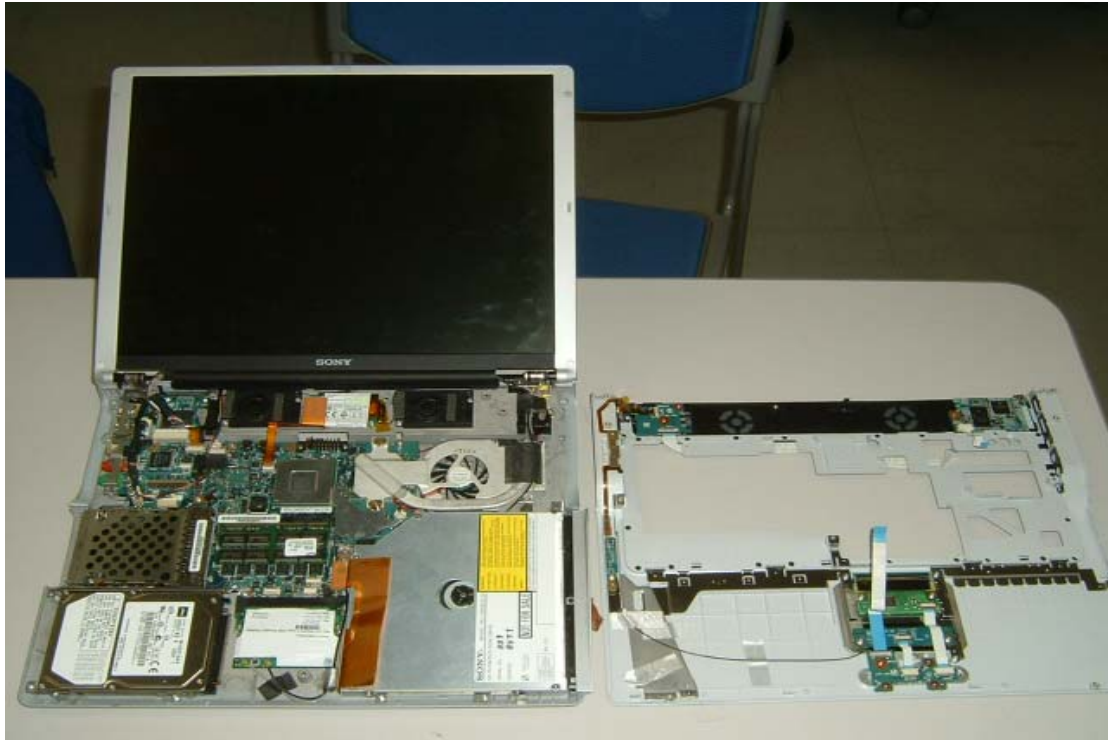
BT Module & W-LAN installed Photo 2
