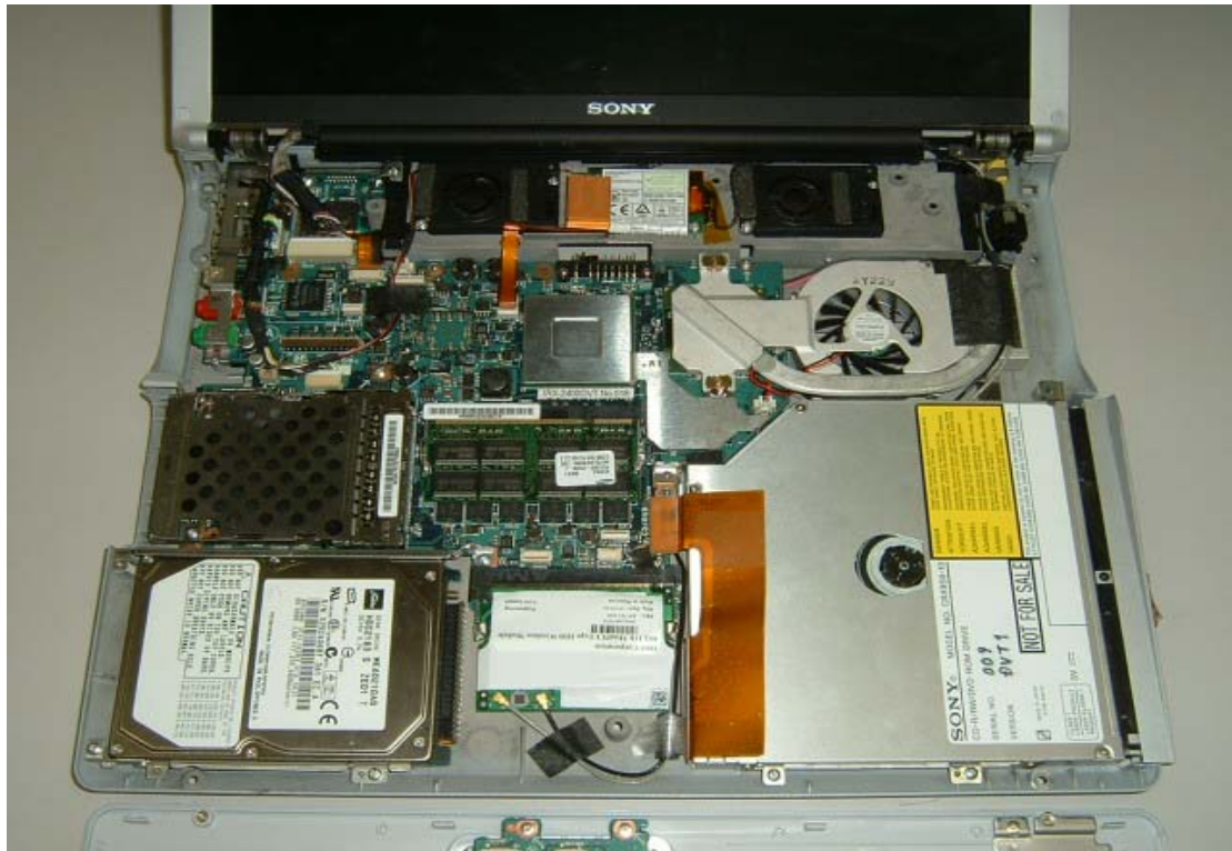
BT Module & W-LAN installed Photo 4
