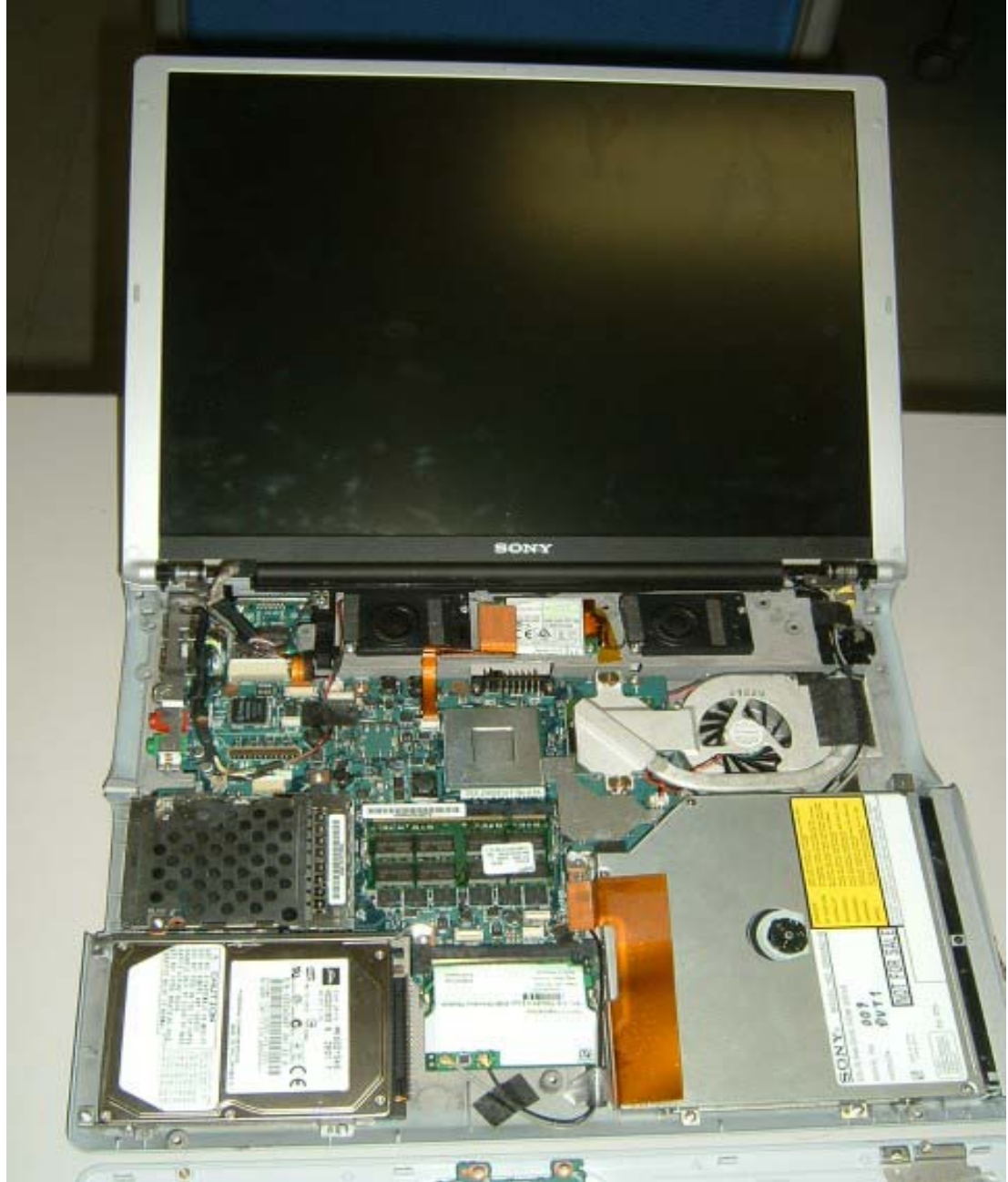
BT Module & W-LAN installed Photo 1
