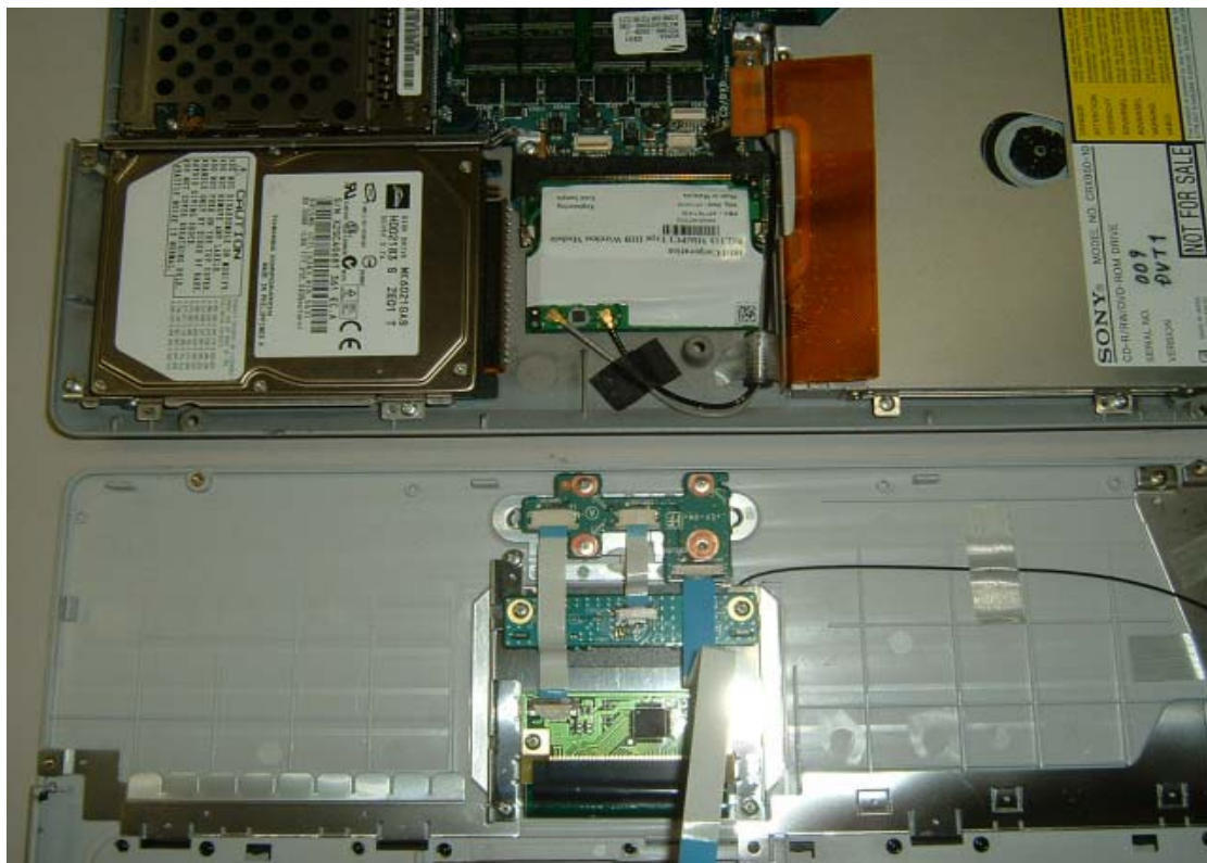
BT Module & W-LAN installed Photo 3
