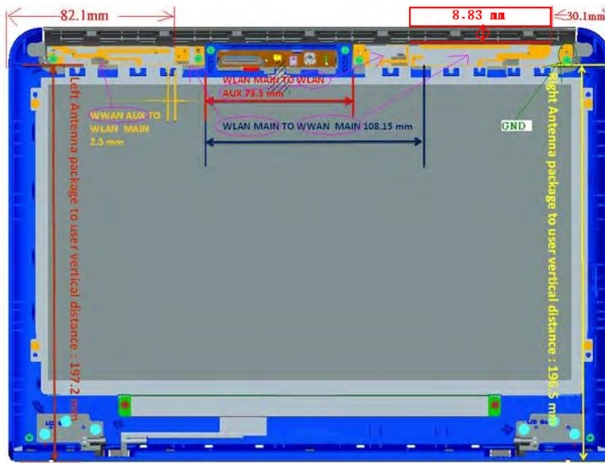
Fig.9 Antenna position of EUT
