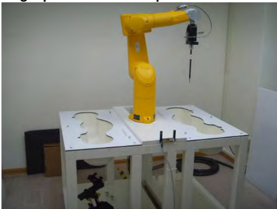
Fig.1 Photograph of the SAR measurement System
