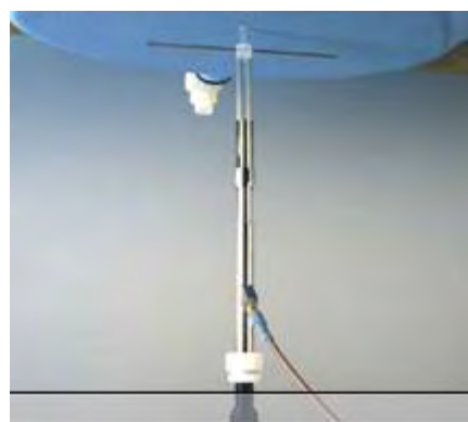
Photograph of the dipole Antenna
