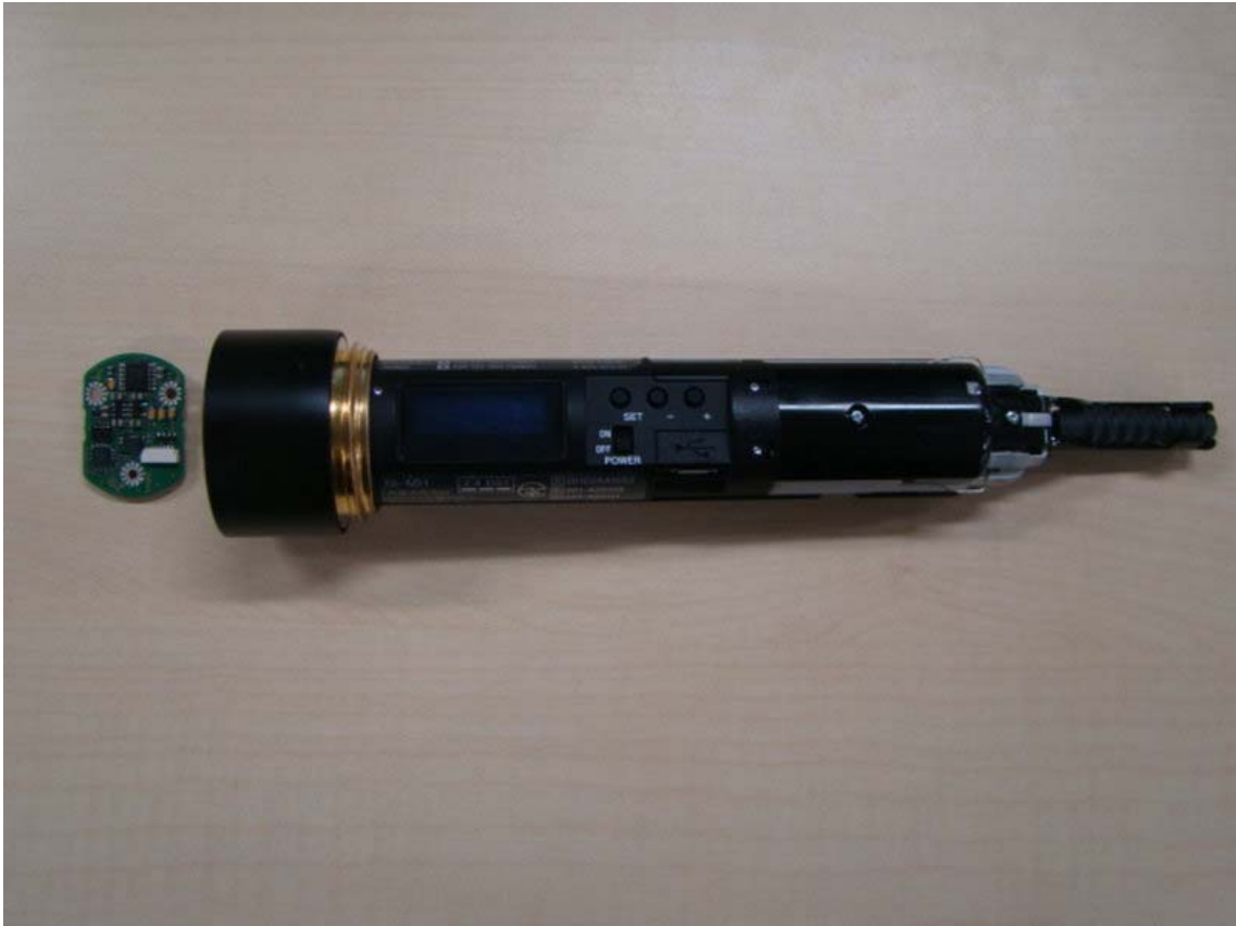
Fig.5: Removed the board AU-356
