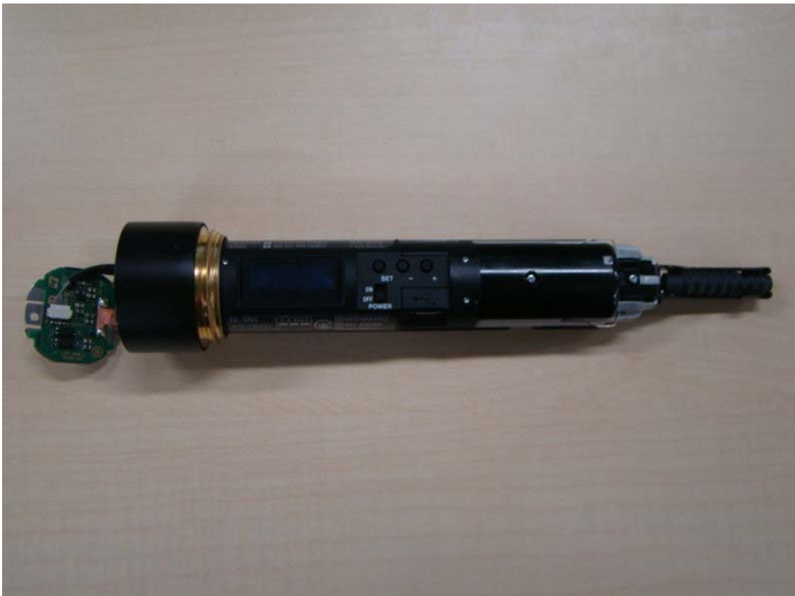
Fig.2: Removed the board CN-3630
