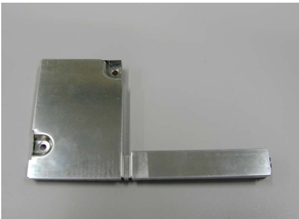
Top View of RF Connector with Shielding
