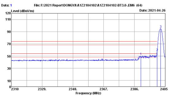
Dis. / Ant. : 3m 2020 MCTD1209-3006 Ant. pol. : VERTICAL Limit : FCC PART 15C PEAK Pressure : 101.7kPa Env. / Ins. : 23.2\*C/52.5% Engineer : Lynn
