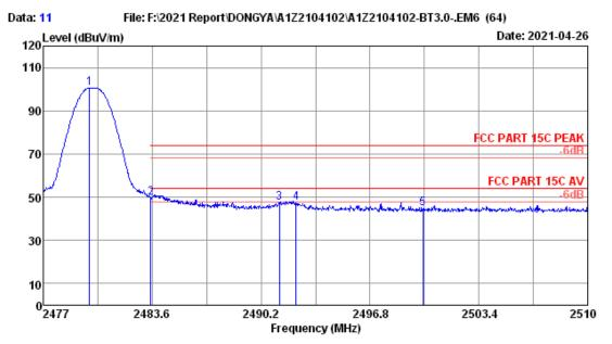
Dis. / Ant. : 3m 2020 MCTD1209-3006 Ant. pol. : HORIZONTAL Limit : FCC PART 15C PEAK Pressure : 101.7kPa Env. / Ins. : 23.2\*C/52.5% Engineer : Lynn
