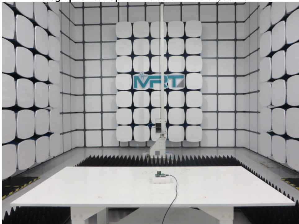
Photograph 2: Set-up for Radiated Emission, above 1GHz
