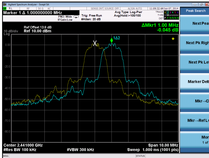
Figure 2: Carrier Frequency Separation-Middle Channel
