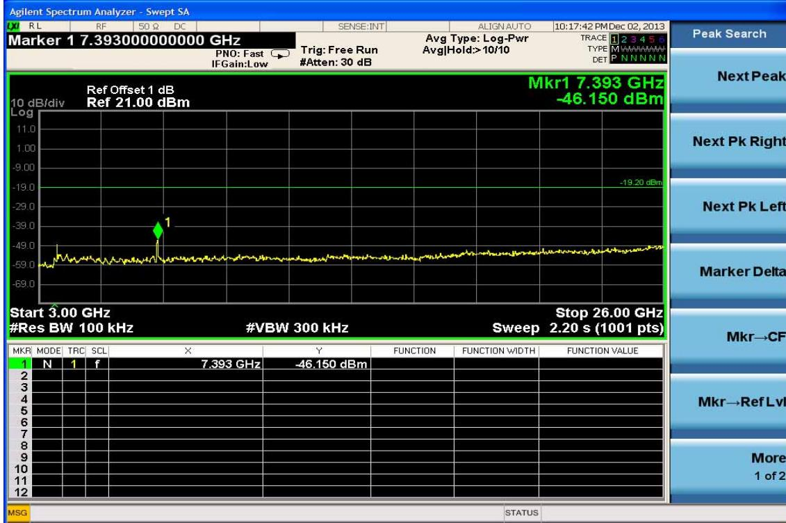
**Conducted Spurious Emission Measurement Result (LE Mode)**
