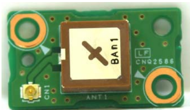
Antenna Top View
