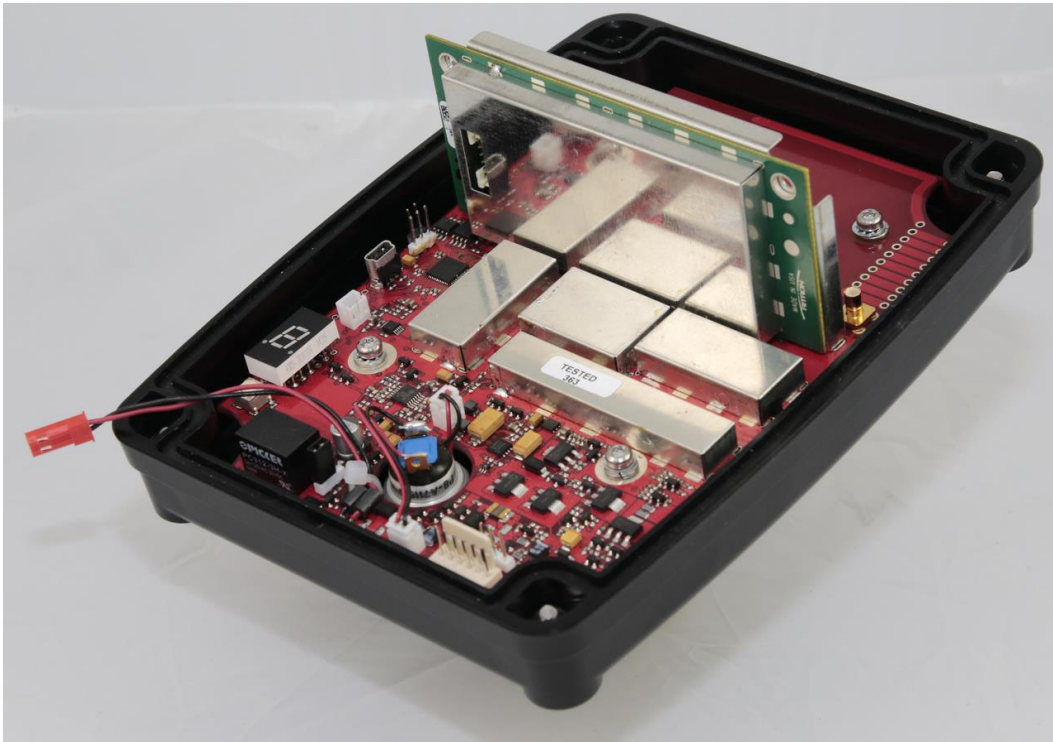
RQX-417DMR w/ 9/RQXD-DMR installed in Front Enclosure
