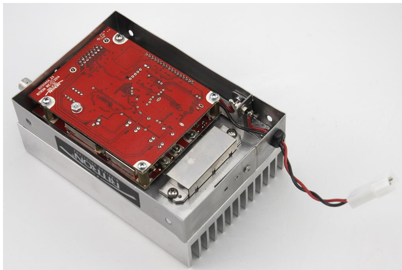
DTX-165-RR-SIG PCB/Heatsink Assembly w/ Enclosure Shield
