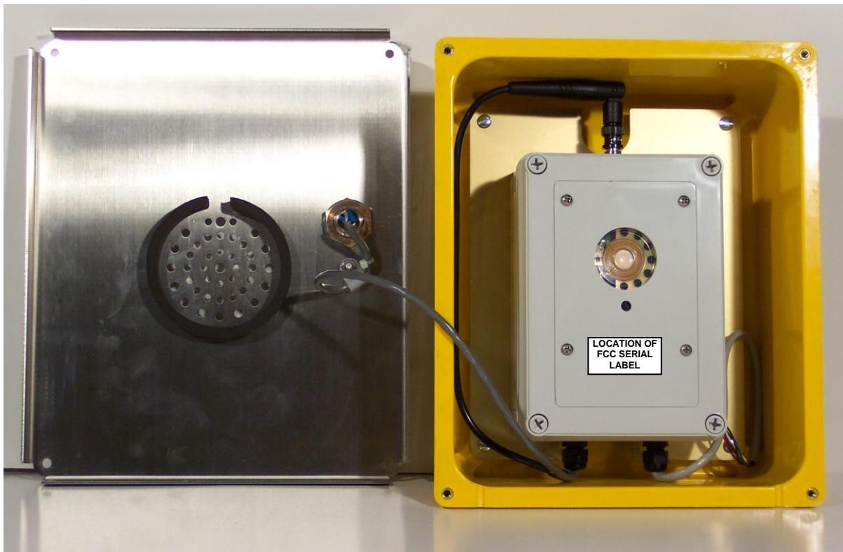
**EXHIBIT:** RQX-156M-XT with ruggedized outside faceplate removed to show location of FCC identification label on the radio case.
