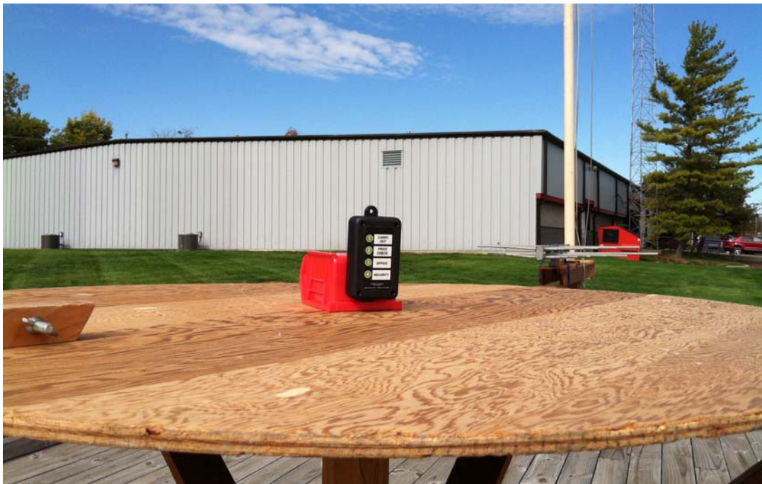
RQA-1B, RQA-4B Radiated Spurious Emissions Test Setup Photos
