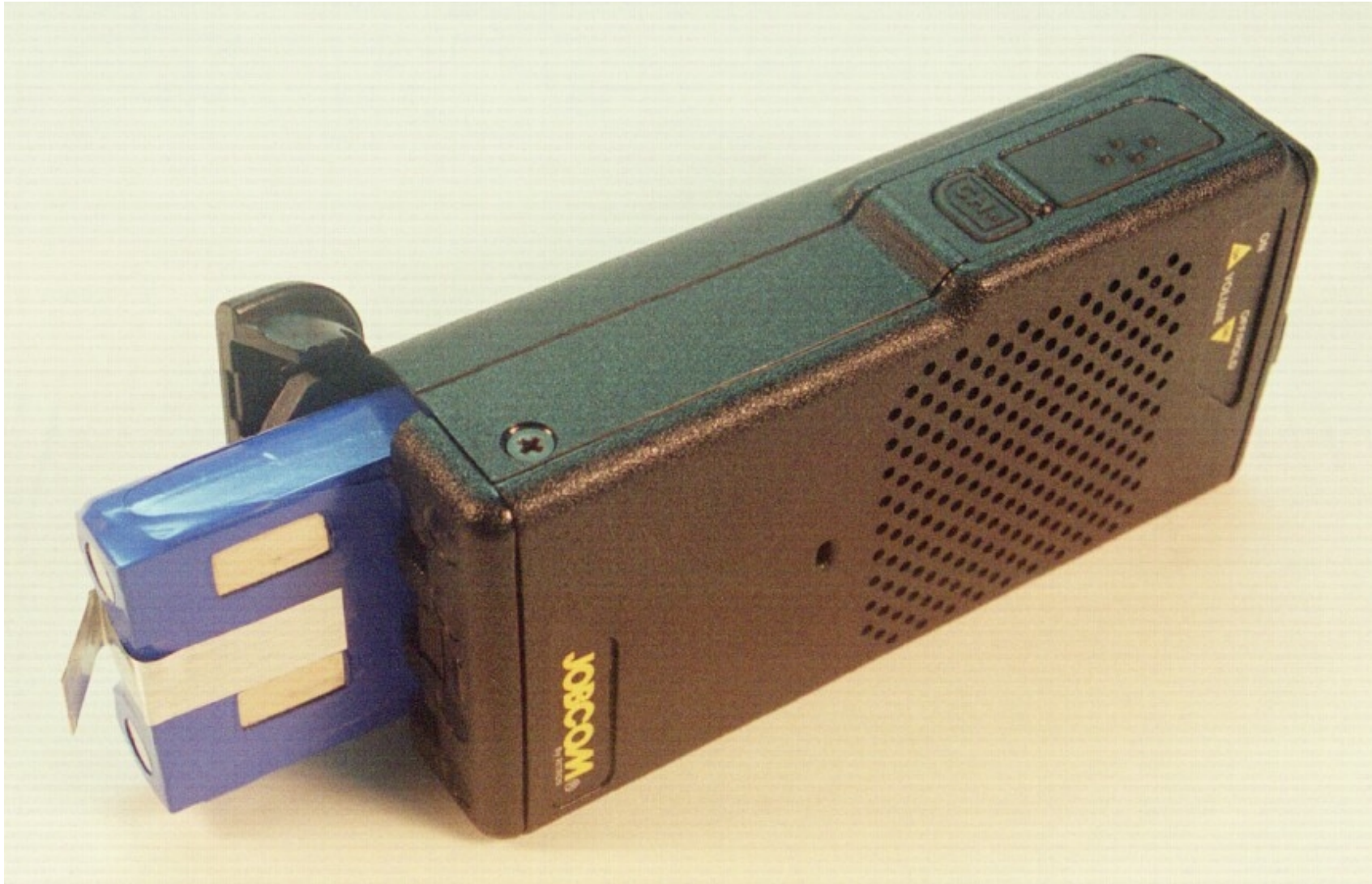
AIERIT13-442 SST-442 battery pack installation into case. PCB assembly, case bottom, and battery insulator must be installed.
