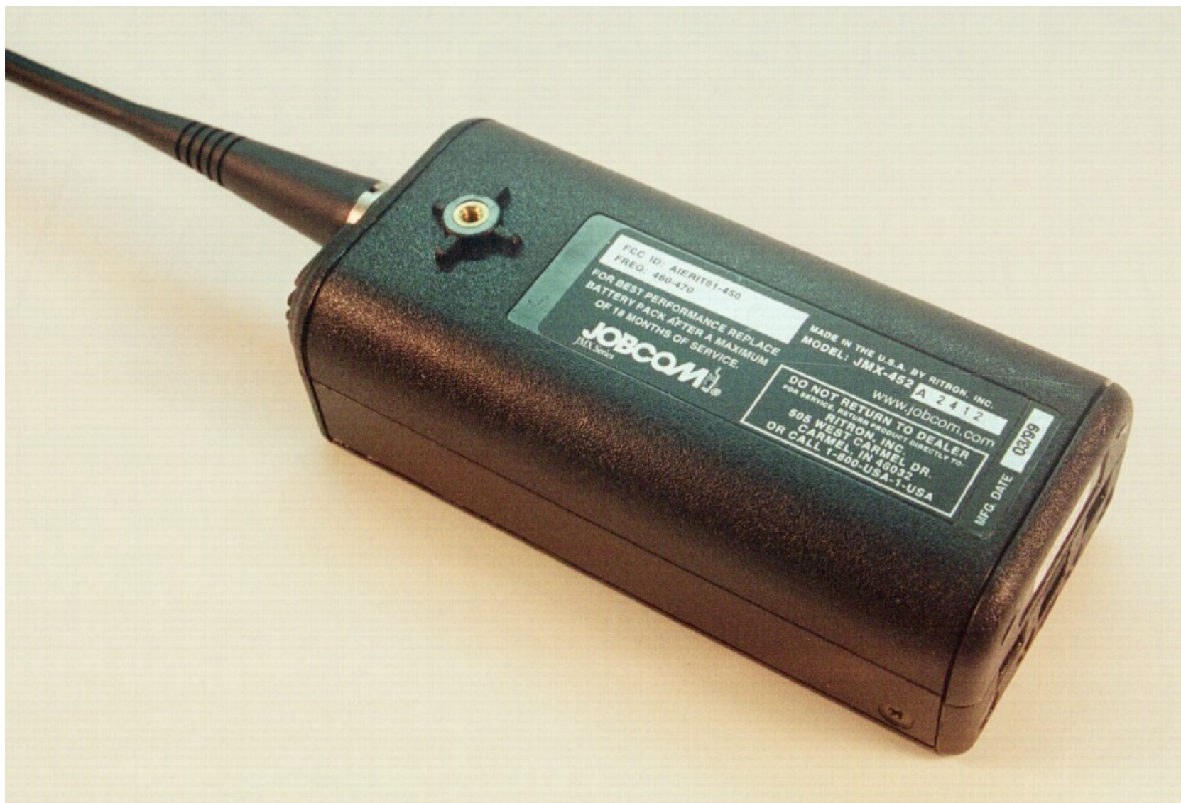
AIERIT13-442 SST-442 case back showing area for FCC identification label and belt clip installation.
