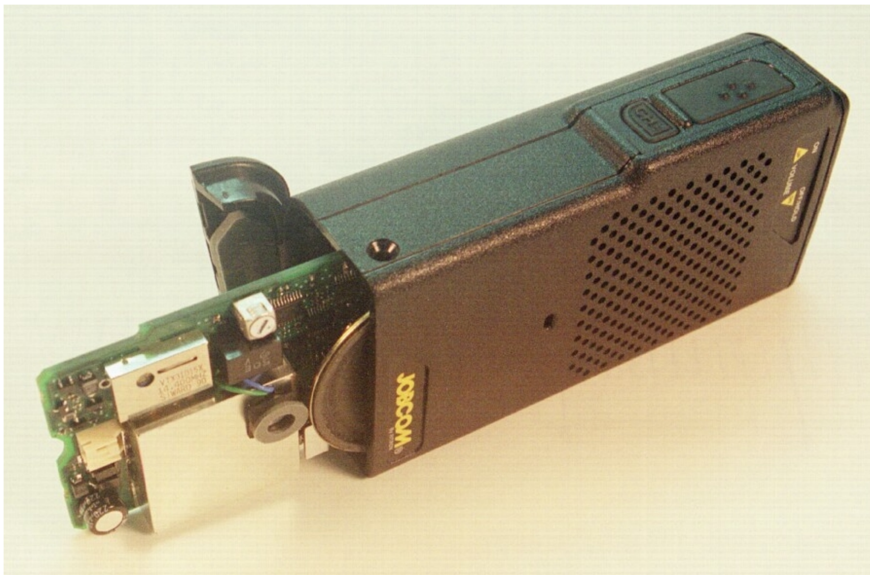
AIERIT13-442 SST-442 PCB installation into case
