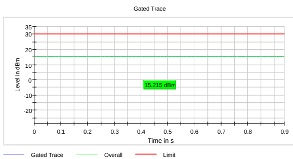
RMS Conducted Power, 5825 MHz, 802.11n, HT20, MCS0, Ant1
