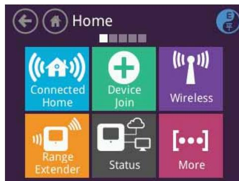
*Note: Almond router does not need any computer or tablet PC for configurations, it can be easily configured via its touch screen panel.*
