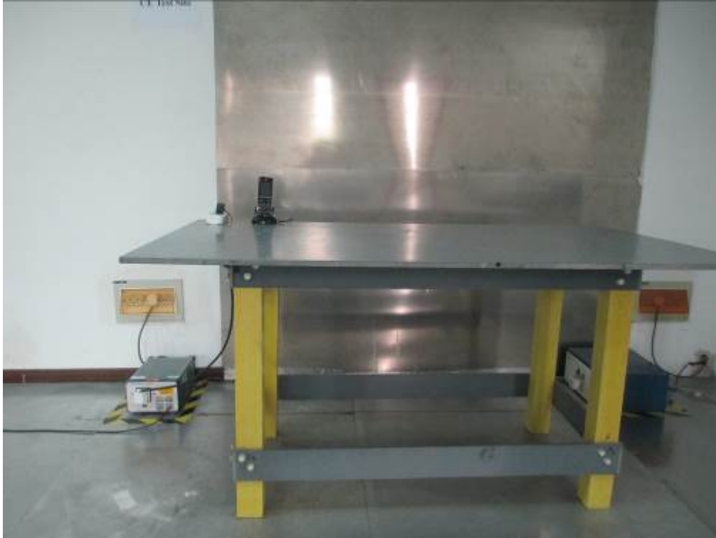
Conducted Emissions Test Setup Front View
