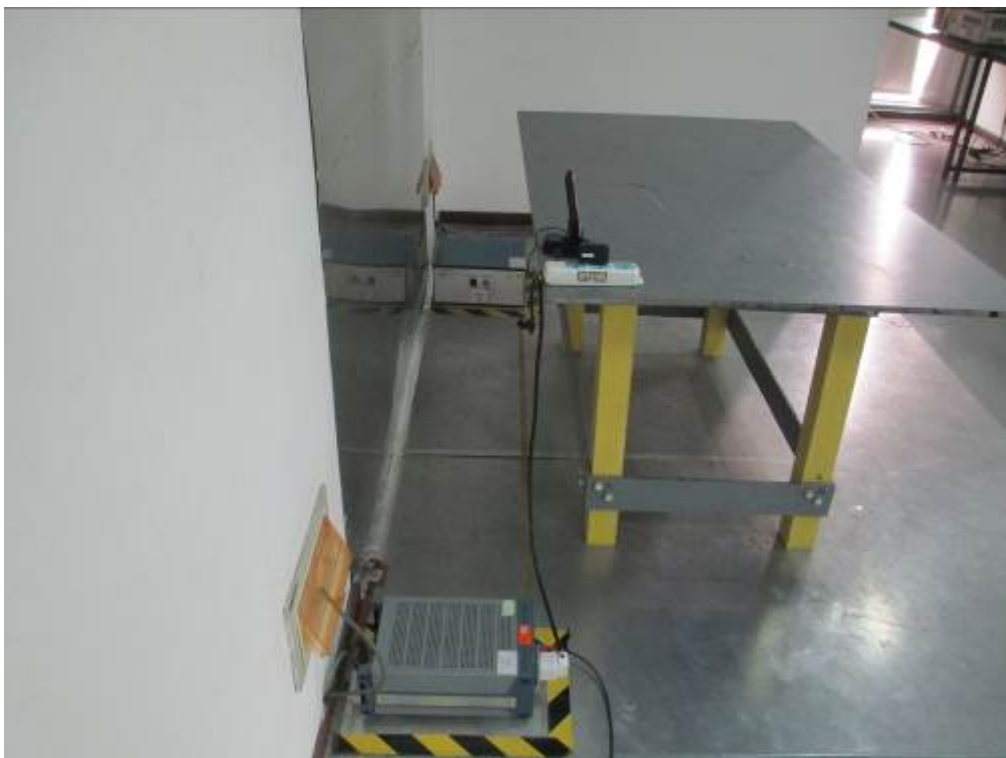
Conducted Emissions Test Setup Side View
