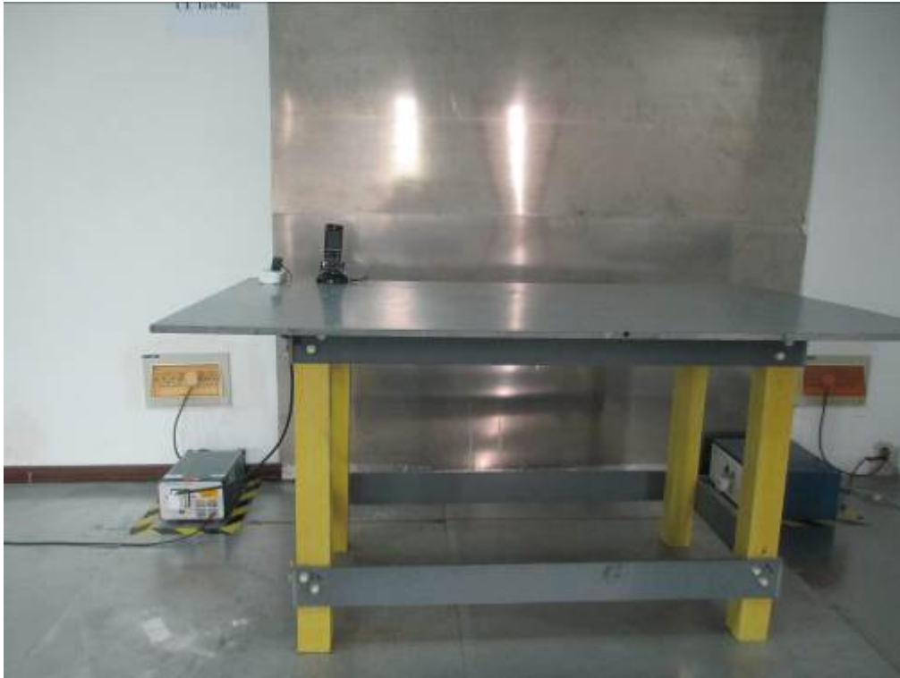
Conducted Emissions Test Setup Front View
