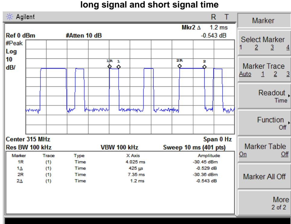
The signal bandwidth was measured and less than 100KHz RBW so PDCF factor is not required.
