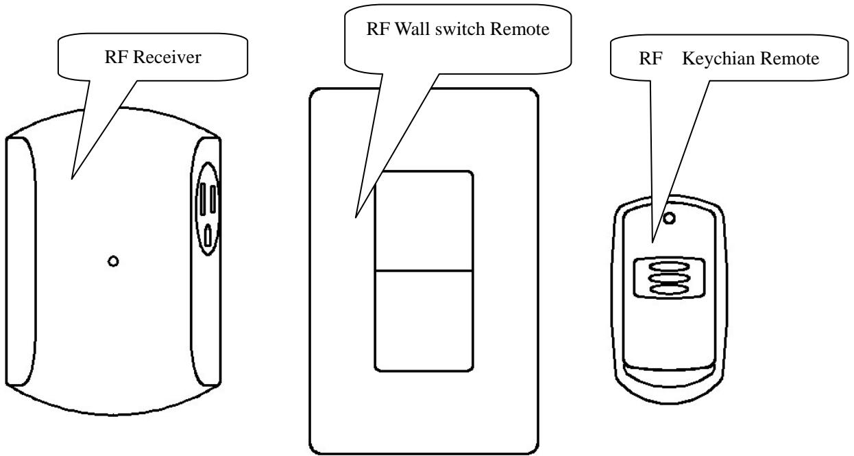
2.1、Wireless radio frequency remote controls are the easiest way to add switched outlet convenience without wiring or the need for an electrician. Simply plug the desired appliance into the receiver and the receiver into any outlet. A press of the handheld transmitter's button turns whatever is plugged into receiver On or Off. Easy handheld transmitter can be taken anywhere or attached to keys.
