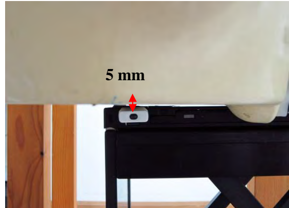
Fig.4 EUT Horizontal down mode to flat phantom
