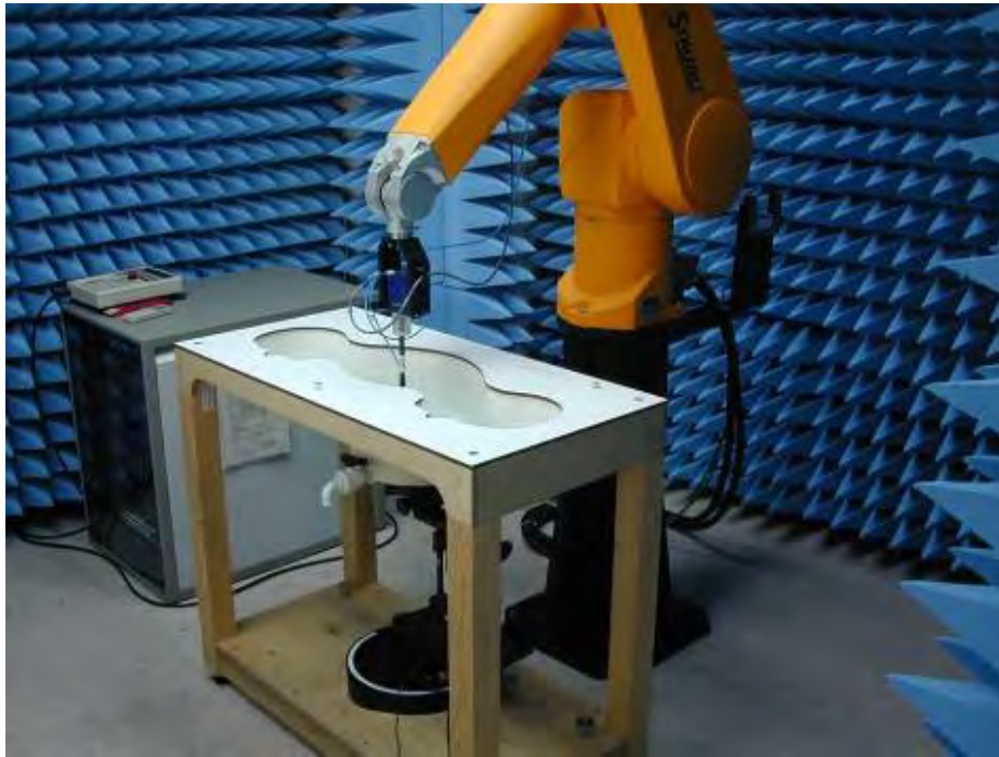
Fig.1 Photograph of the SAR measurement System
