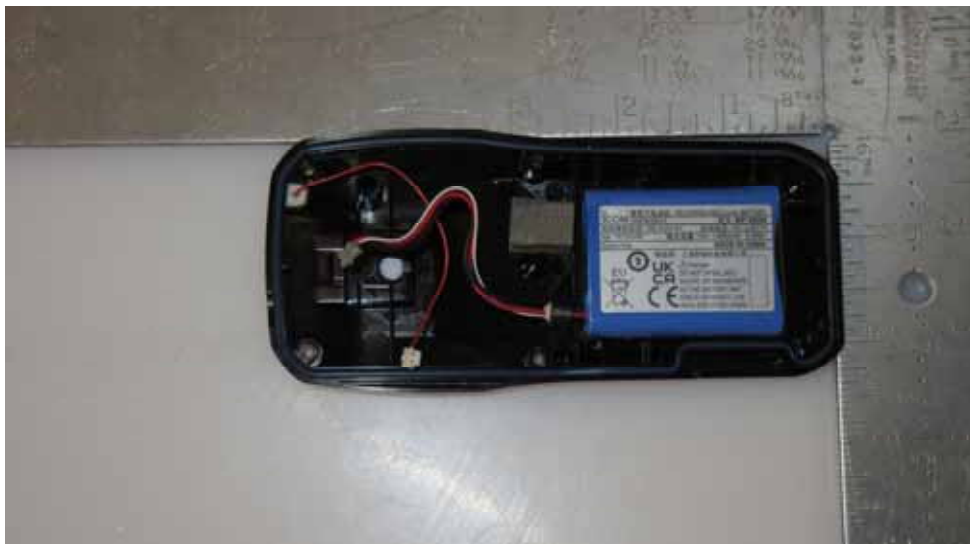
<Li-ion Chargeable Battery (BP-282N, 3.6V, 1570mAh)>
