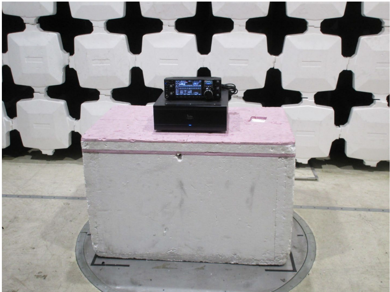
Radiated Testing, Table Setup #1
