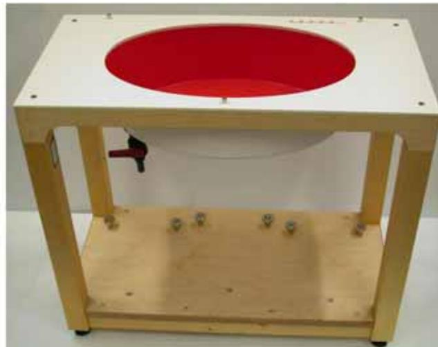
For body mounted and frontal held push-to-talk devices, an IEC 62209-2 compliant Oval Flat Phantom (ELI 4.0) with a base plate thickness of 2mm is used.
