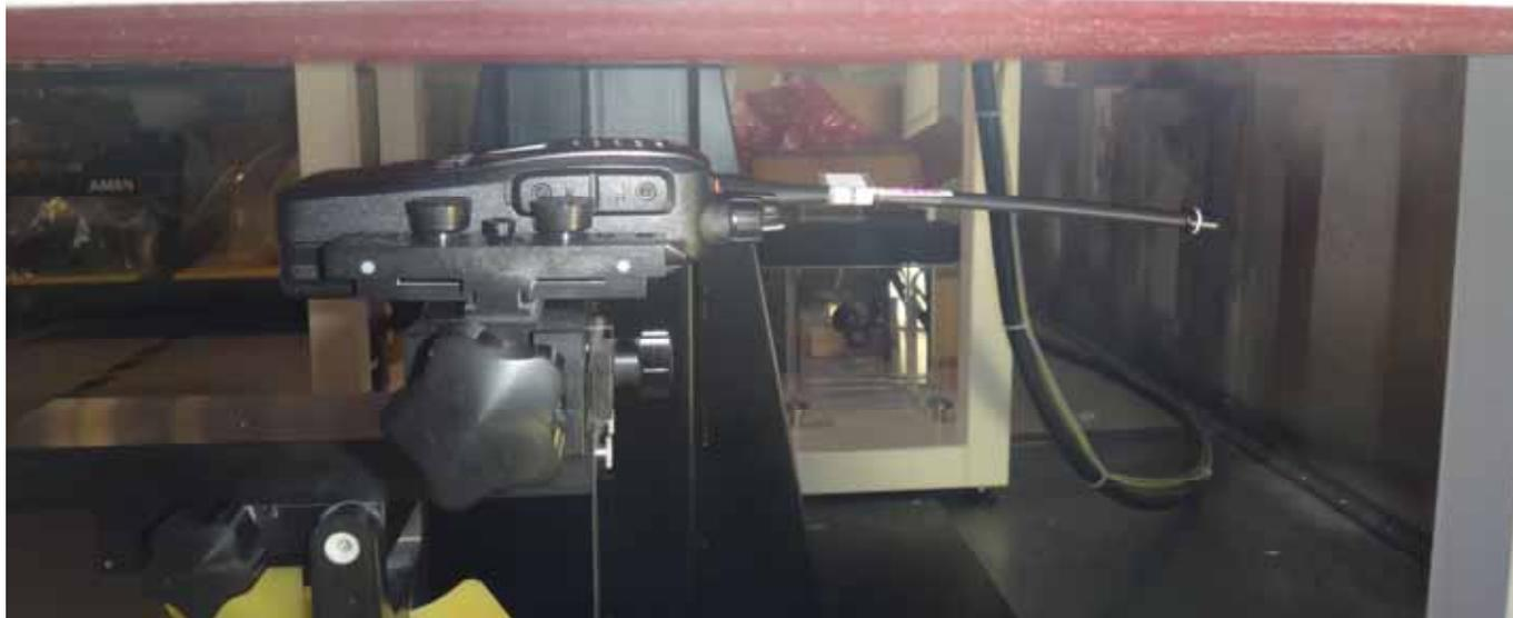
**<Face Frontal Position, FA-SC61UC Antenna, BP-280 battery pack>**
