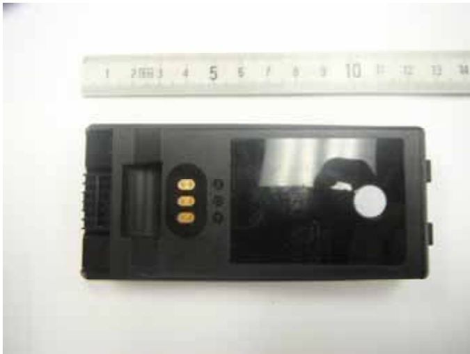
Li-ion Chargeable Battery (M/N: BP-284 Li-ion, 7.2V, 3210mAh)
