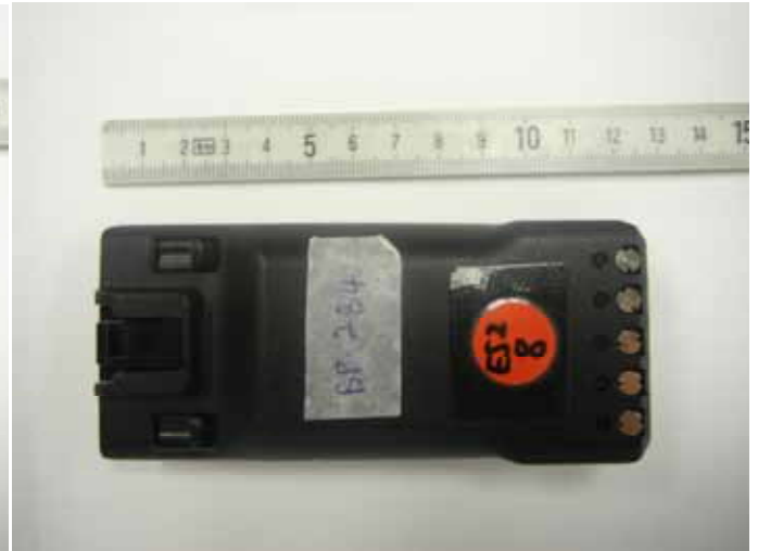
Li-ion Chargeable Battery (M/N: BP-284 Li-ion, 7.2V, 3210mAh)
